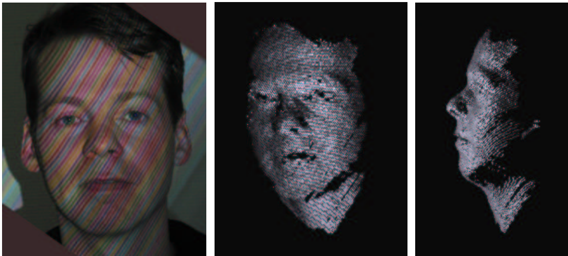
Figure 38: Striped image and 3D representations from extracted 3D data
