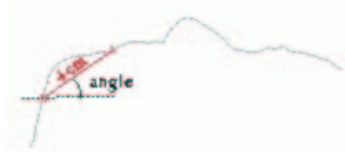
Figure 49: slope measurement along the profile
