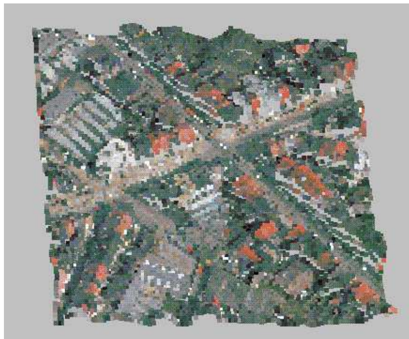
Figure 4.32: 3D model with colors: energy minimization result, potential functions - truncated quadratic, \alpha = 2 .
