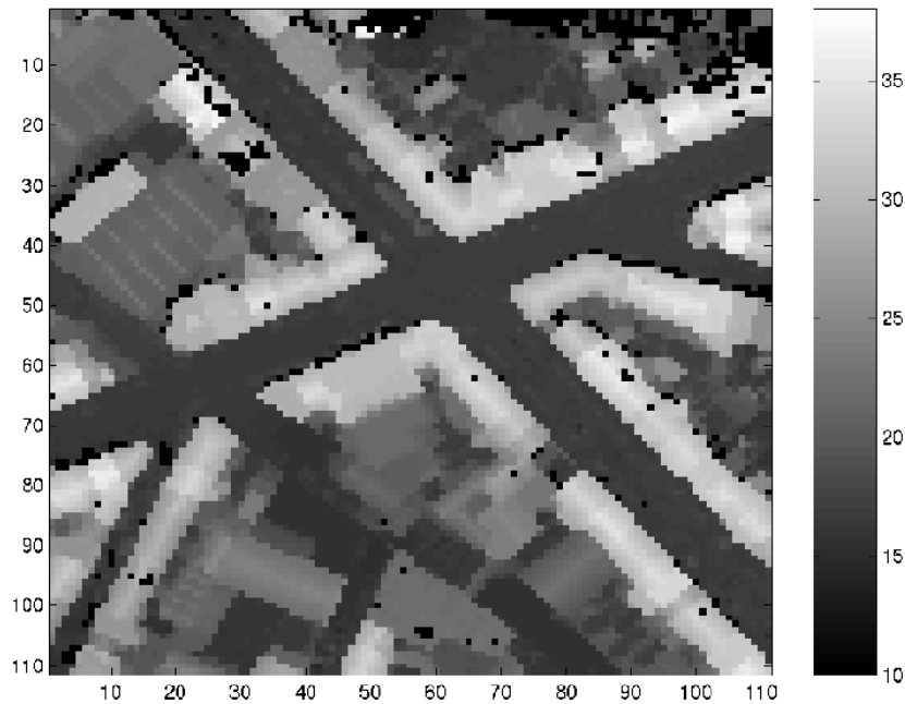
Figure 4.13: DEM obtained from stereo photos. The sampled version to adapt the resolution (1.8 meters) for comparisons. Black color corresponds to pixels where altitude values are not determined.
