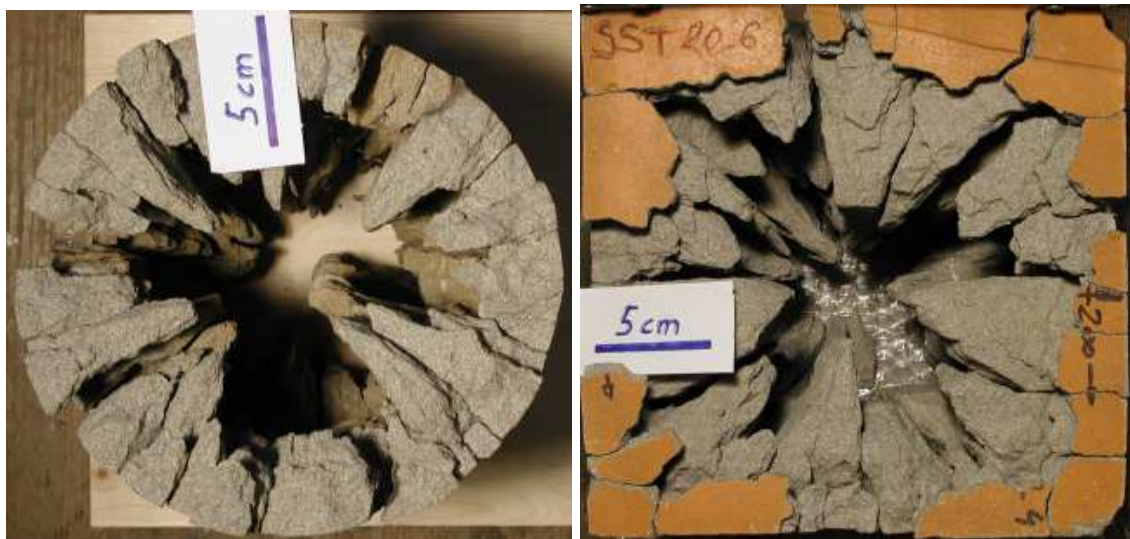
Figure III.1: Rebuilt cylindrical and cubical samples
