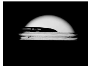
Fig. 9. Picture of a centimetric polymerized silicon drop taken from the side (about 0.5 mm thick).
