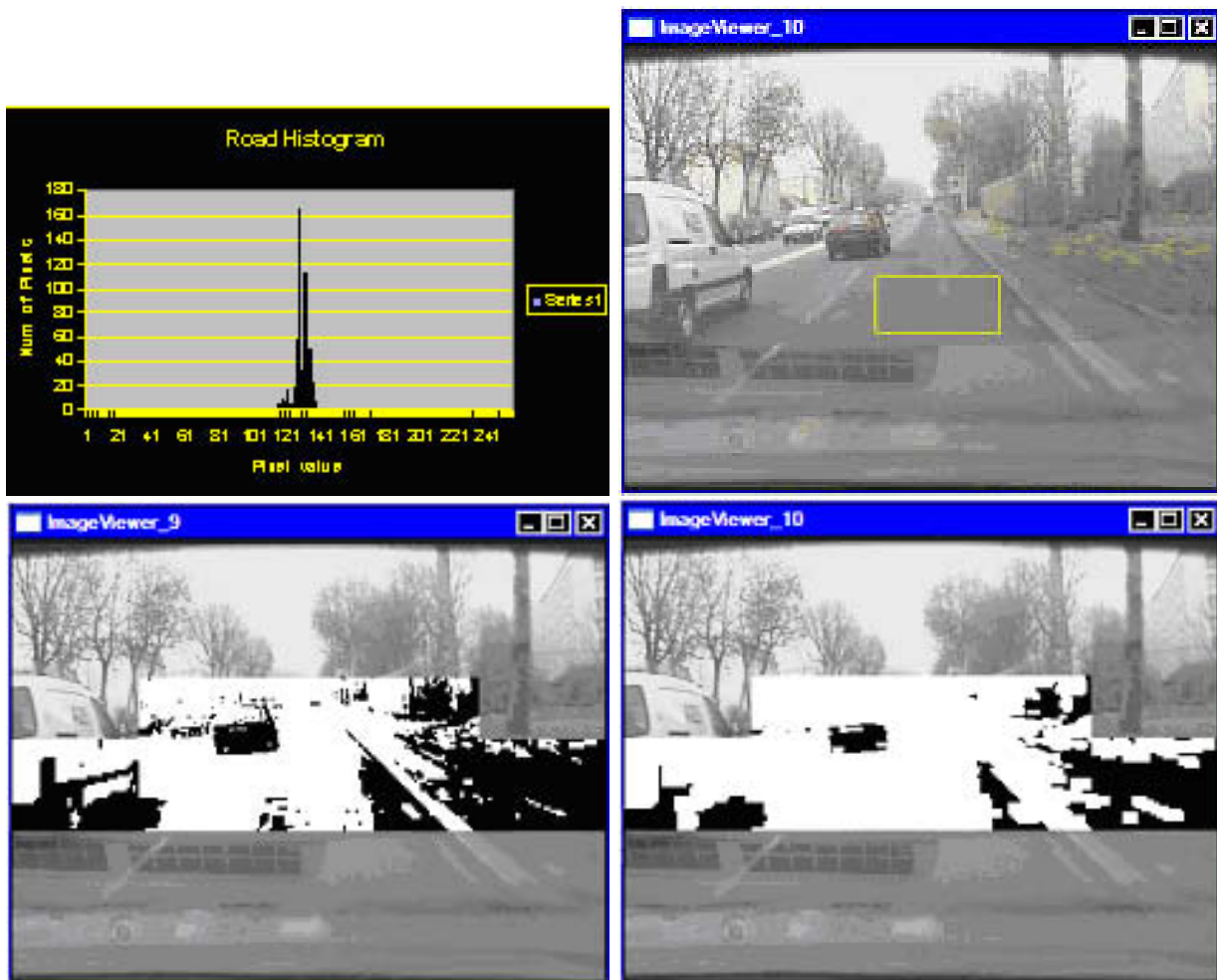
FIG. 6.8 – The shadow detection algorithm. The histogram (top left) is calculated on the road rectangle (top right). The image is thresholded (bottom left) and later eroded (bottom right).
