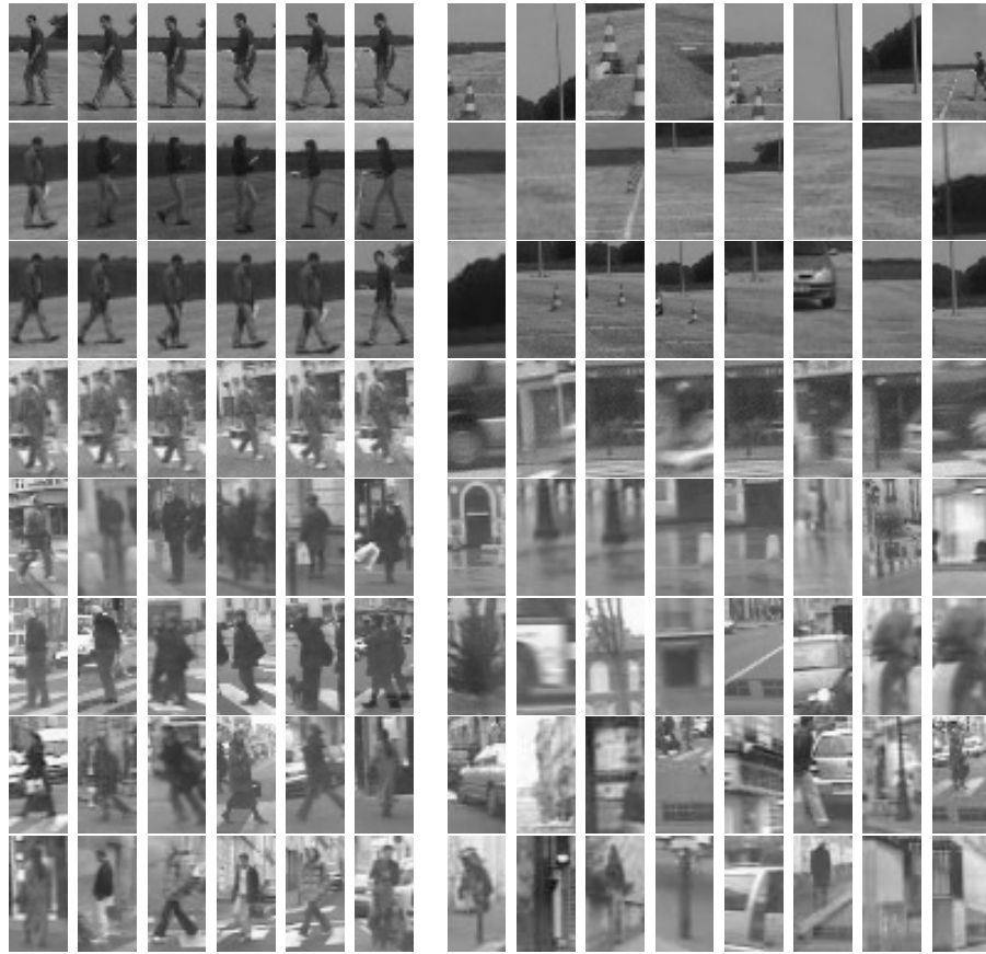
FIG. 3.43 – Positive (left) and negative (right) examples for the different steps (each line is a step, from top to bottom). These examples received the minimal (for positive examples) or maximal (for negative examples) score during classification in their respective step.
