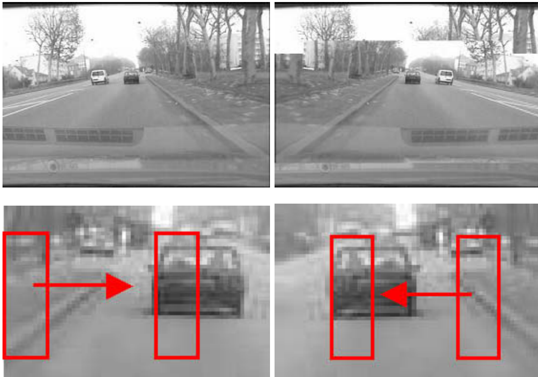
FIG. 6.11 – The Symmetry detection. From top to bottom : the original image, the mirrored image, left and right rectangles.
