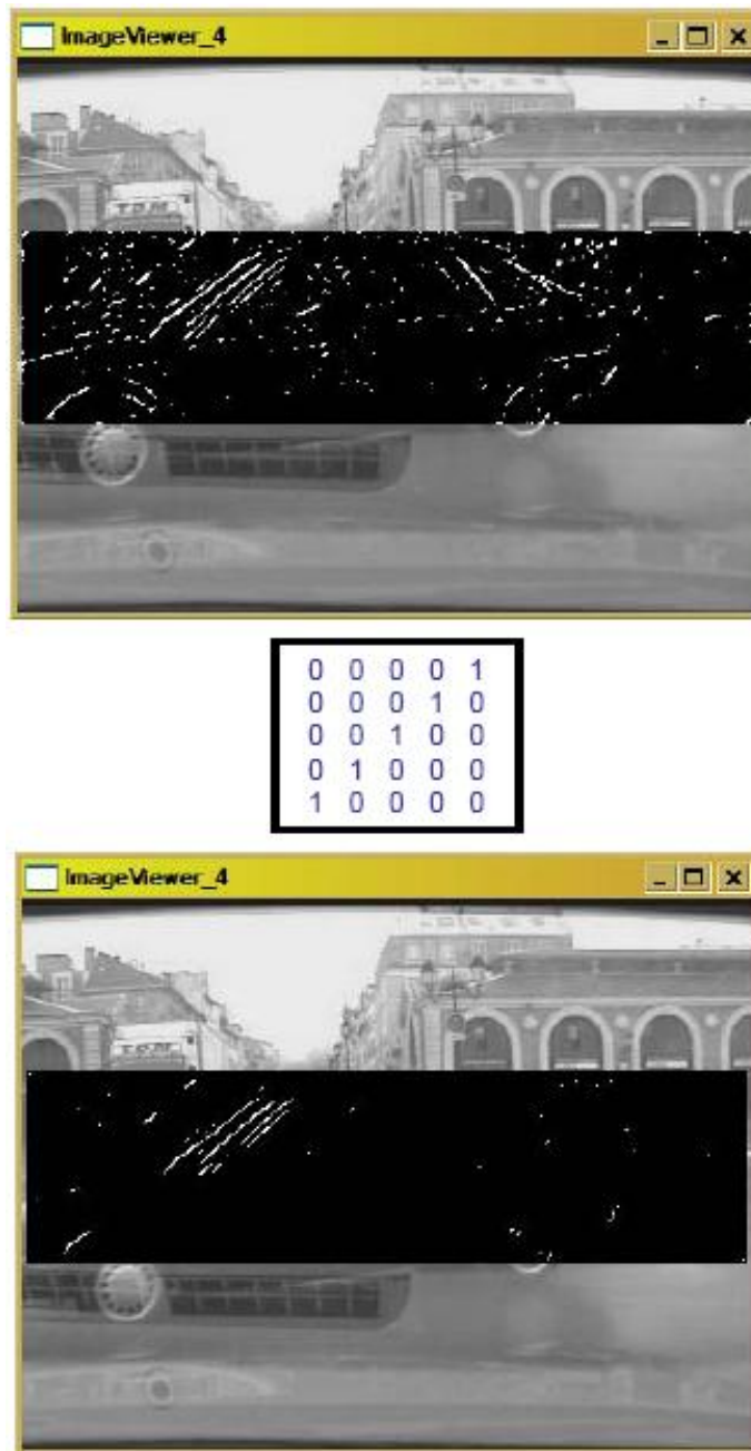
FIG. 7.9 – The result of linear filtering with the left diagonals (upper image) still contains many right diagonals, due to the strong edges to the closely-passing car. After erosion with a simple 5x5 diagonal element (in the middle), we get a better image without right diagonals (lower image).
