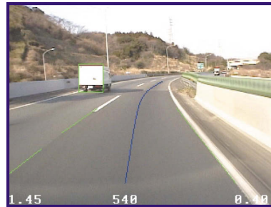
FIG. 2.10 – The lane departure warning system of MobilEye (source : Mobileye's website)
