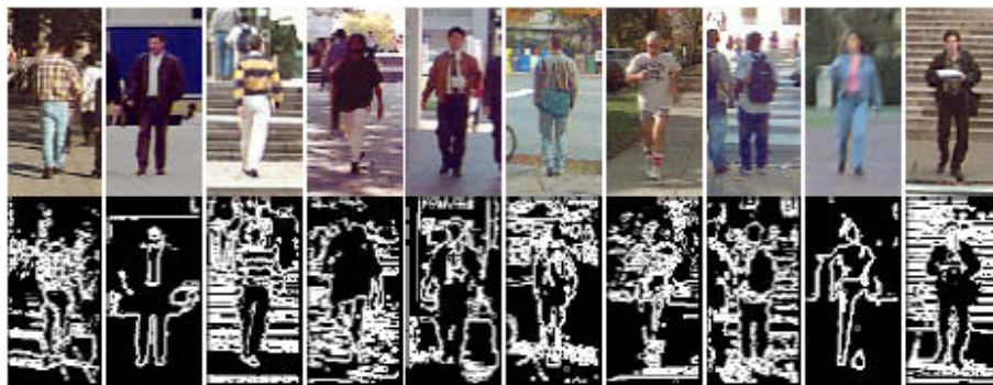
FIG. 3.3 – The top row shows examples of images of pedestrians in the training database of Papageorgiou et al. The examples vary greatly in color, texture, and background. The bottom row shows the corresponding edge maps generated by a Sobel filter
