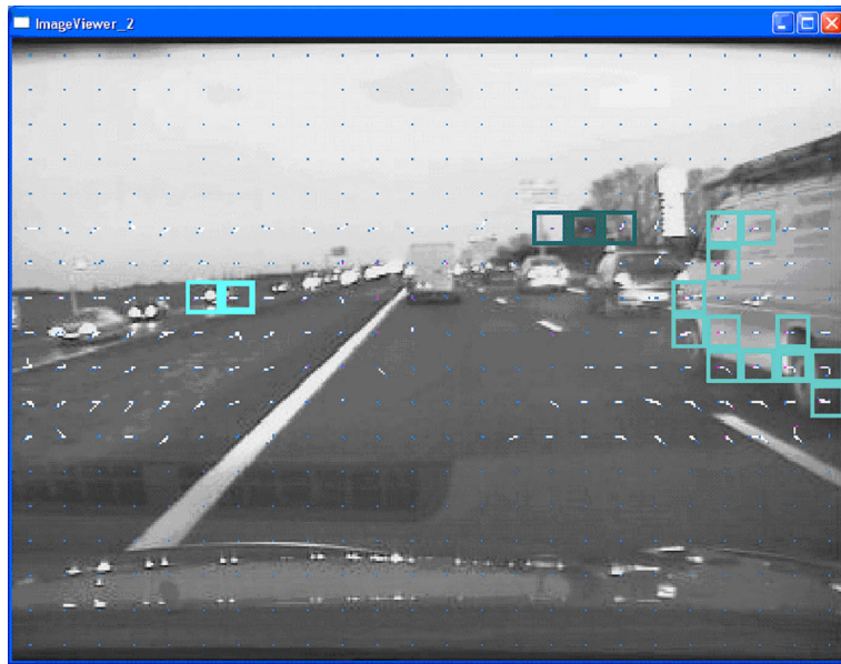
FIG. 4.4 – The car entering on the right appears only by its exterior. The interior blocks are not unique, therefore are not considered as having valuable information.
