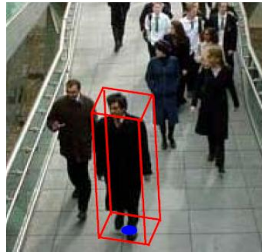
FIG. 7.3 – The box of a pedestrian, and its origin in the bottom centre point.
