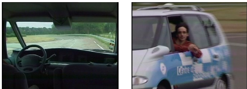
FIG. 2.14 – Automatic vehicle guidance presented by the Center of Robotics of École des Mines de Paris, in IV2002 using vision. In the second image, we can see the driver’s hands outside of the car, while the car is driving at about 50 km/h on curve.
