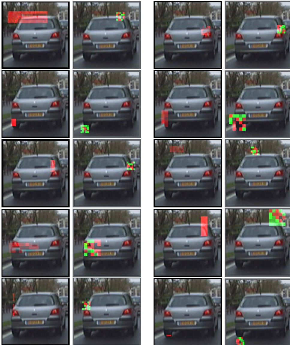
FIG. 3.24 – 10 examples of the 5 \times 5 feature, learned for car detection. Each feature is brought in a pair of images (in two columns). On the left of each pair, we have drawn the intensity that this feature responds on that particular image. On the right, we see the 5 \times 5 array of the feature, drawn on the spot where it gives the maximum response for that image.
