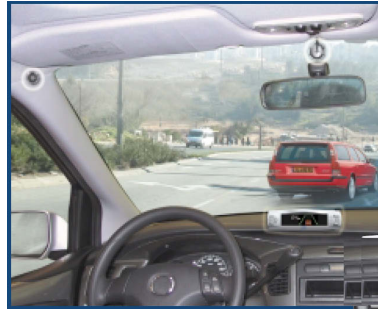
FIG. 2.11 – The forward collision warning of MobilEye (source : Mobileye's website)
