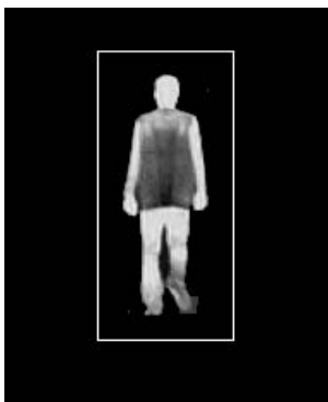
FIG. 3.1 – The pedestrian conventions : the detection window's height is twice as large as its width, and the pedestrian leaves margins of about 10%.
