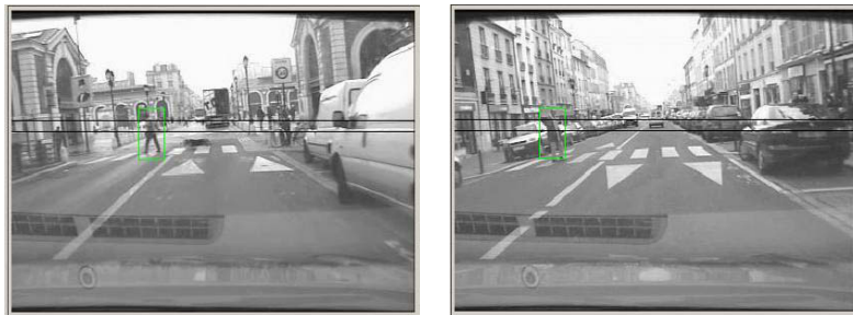
FIG. 3.42 – Results of the classifier in step 8 on two independent test sequences.
