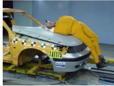
FIG. 2.9 – Front cover which is opening to reduce pedestrian impact
