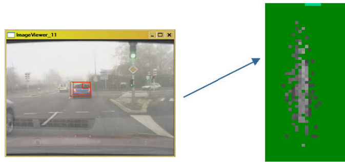
FIG. 6.3 – A typical vehicle target, frontal image (left) and its particles on a bird's eye view (right).
