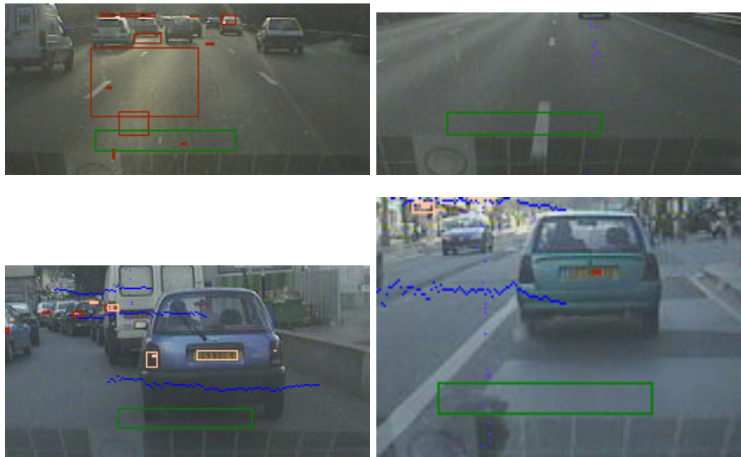
FIG. 6.14 – Examples for cases where the shadow rectangle do not provide a homogenous histogram.
