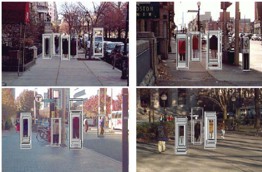
FIG. 3.6 – Results from the pedestrian detection system of Papageorgiou et al.
