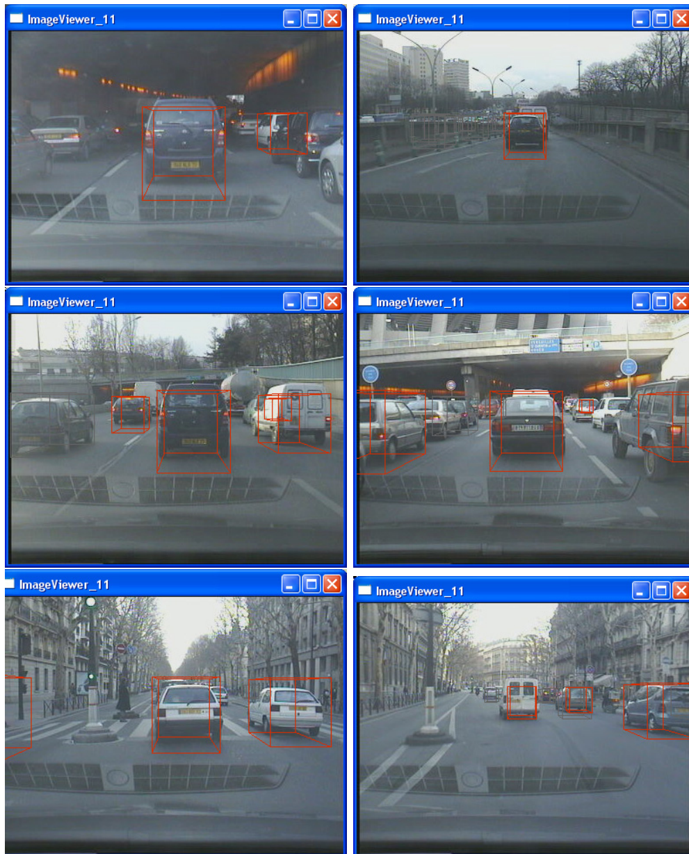
FIG. 6.32 – Successful detections in a variety of conditions.
