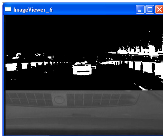
FIG. 6.17 – Shadows which might resemble a vehicle without the two-bases test.
