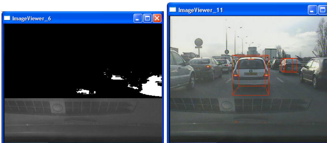
FIG. 6.22 – The shadow shape of a cut-in vehicle.
