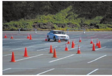
FIG. 2.17 – Fully automated LeSabre on test track : lateral control
