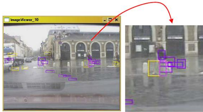
FIG. 7.6 – The left diagonals in the image are marked with a purple rectangle, while the right diagonals are marked with yellow ones. The intersection between the two is marked by a pink triangle - and this exists only in the area of the legs of the pedestrian.
