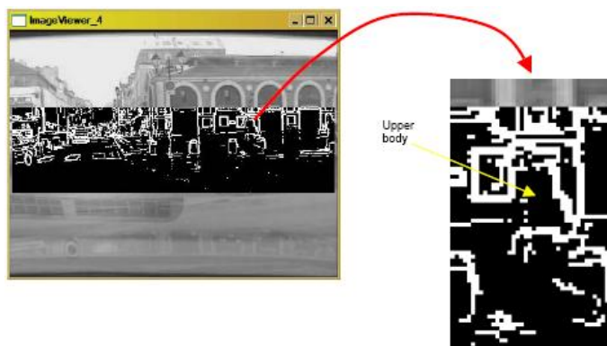
FIG. 7.11 – A typical pedestrian in an edges image. In the zoomed part on the right we see that indeed the upper body of the pedestrian is characterized by a "hole" block whereas the outline of this body part has some edges.
