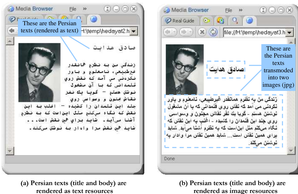
Figure 5.9: Screenshot of the adapted content of Figure 5.8 for a) a terminal supporting Persian character set, and b) a terminal with no Persian character set support.
