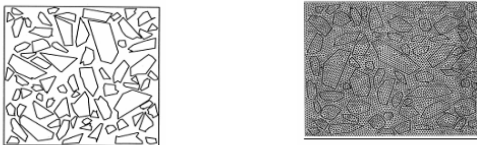
Figure 2-19. Finite element mesh generated (thick lines represent interface elements).
