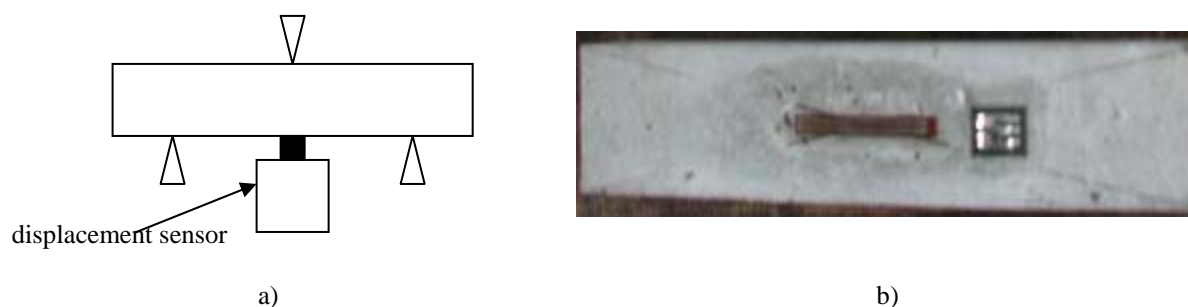
Figure 4-9.a) Displacement sensor; b) Strain gauge is located horizontally on the concrete beam for the three point bending test.
