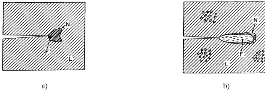
Figure 7-7. Non-linear behavior in a) brittle-ductile material, b) quasi-brittle material (concrete) L: linear behavior, N: non-linear behavior, f: fracture process zone [Bazant et al. 2002]
