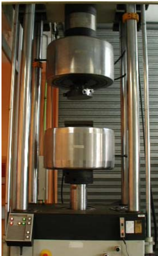
Figure 4-10. left) 100 t. press, type INSTRON 8505 (compression test); right) 15 t. press type INSTRON 8500.
