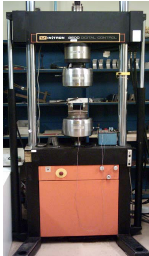
Figure 4-10. left) 100 t. press, type INSTRON 8505 (compression test); right) 15 t. press type INSTRON 8500.
