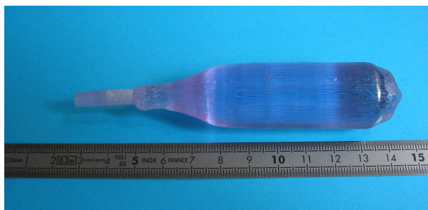
Figure 12. Cristal SrGdGa 3 O 7 :Nd 2%.
