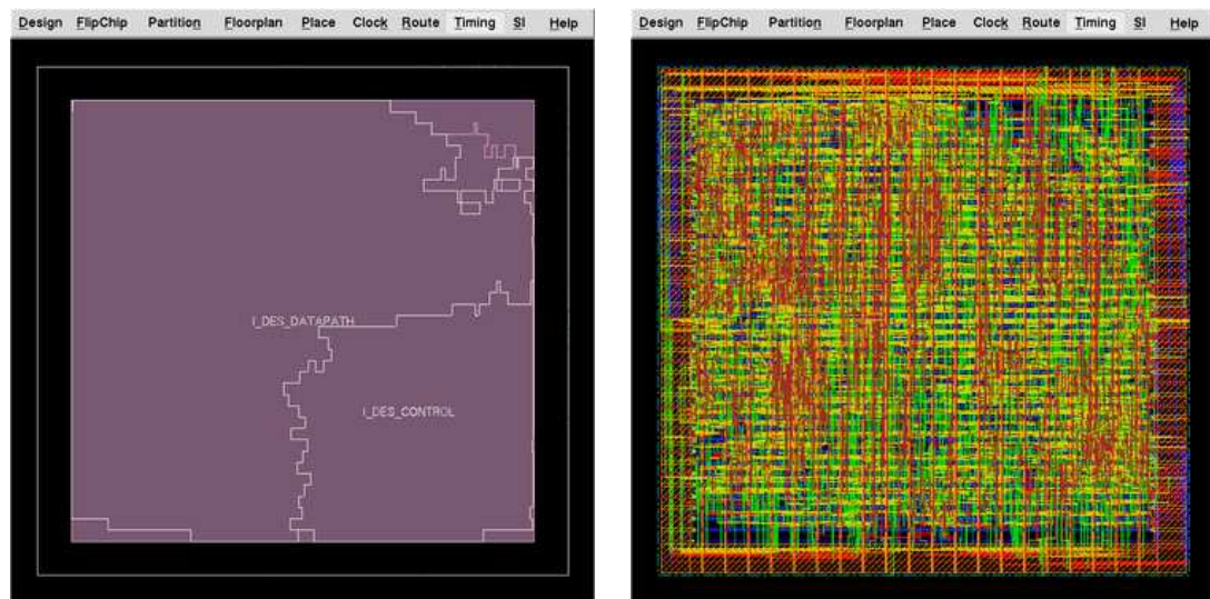
Figure 3.11: The multi-mode DES after place-and-run in 130 nm technology. Left : Datapath / Control partitioning; Right : Final layout.
