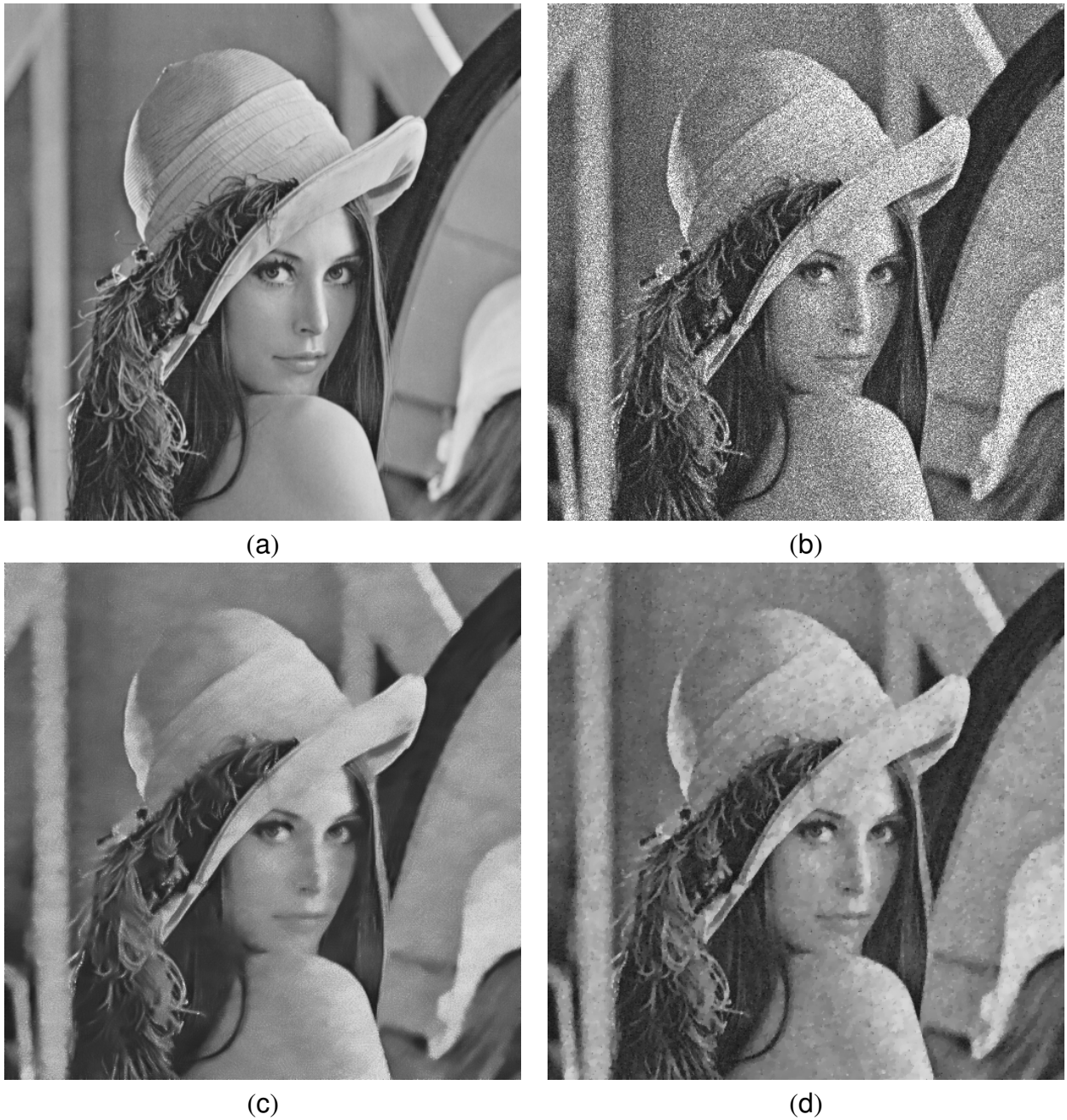
Fig. 4.10: (a) Original Lena image (b) image corrupted by speckle noise with variance \sigma_n = 0.025 (c) Random walk based restoration result (d) Total variation minimizing based restoration [7]
