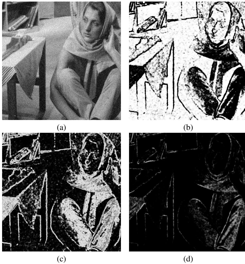
Fig. 3.6: Results of an image partition: (a) original noisy image ( \sigma_n=20 ), and conditional probability function relative to (b) "smooth component" p(o_x|smooth) , (c) "texture" p(o_x|tex) and (d) "edges" p(o_x|edge)
