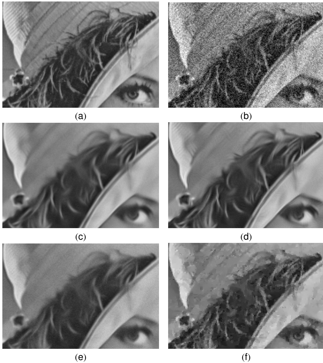
Fig. 5.8: Zoom on the Lena image (a) Original image, (b) Noisy image (c) Our method using fixed bandwidth (d) Our method using variable bandwidth (e) Non local functional minimizing (5.9) (f) Total variation minimizing with variable local constraint
