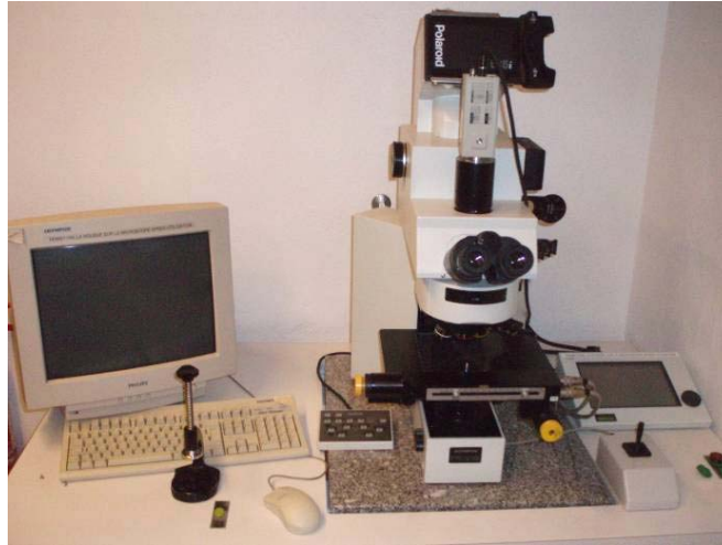
Figure II.46: Microscope optique Olympus AX70.
