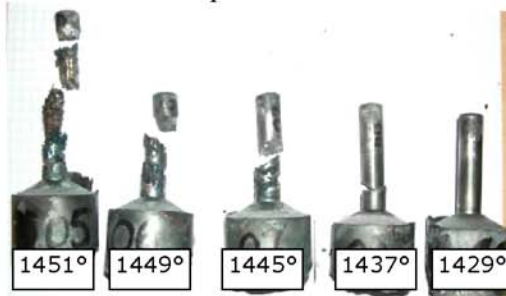
Figure 4. Parts obtained by decreasing the initial temperature of the slug.
