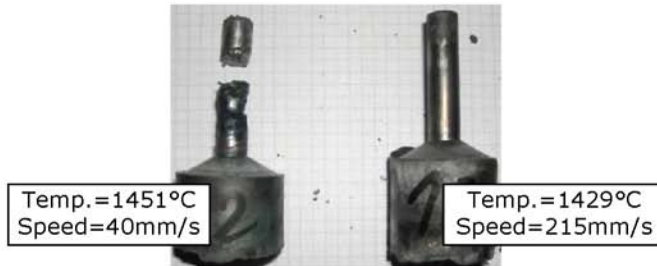
Figure 6. Two parts obtained with the same force (200kN)
