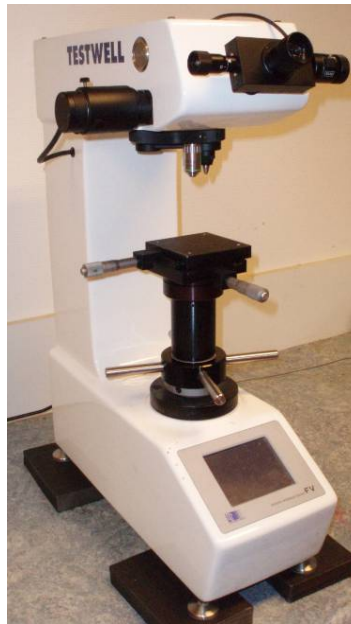
Figure II.48: Machine de microdureté FV70 Future-Tech corp.
