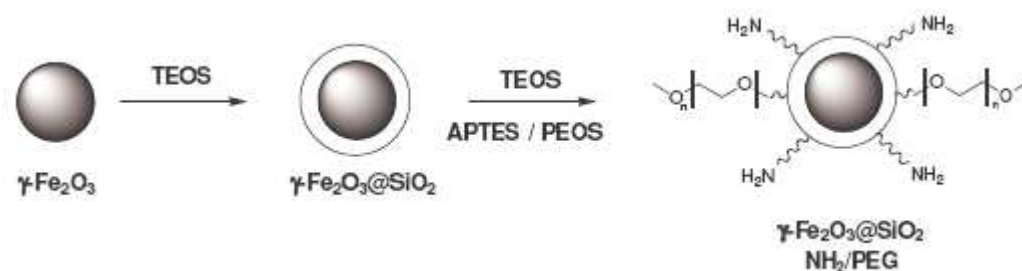
Figure 1: Reaction scheme of the synthesis of the nanometric bifunctional maghemite/silica core/shell particles
