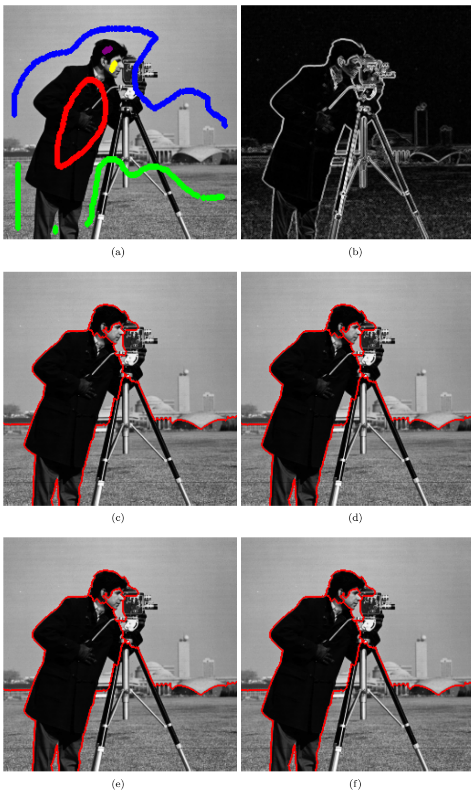
Figure 5.8: Watershed Segmentation. (a) Original image (256x256) surimposed with the markers. (b) Morphological gradient. (c) Minimal spanning forest of the flooding distance. (d) Bi-criteria shortest path forest. (e) Lexicographical shortest path forest. (f) Watershed using Meyer's algorithm based on hierarchical queues.
