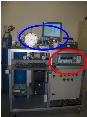
Figure 2.13. Photo of the primary standard (Blue circle: volumes zoomed in Figure 2.14; red circle: photo-acoustic spectrometer)
