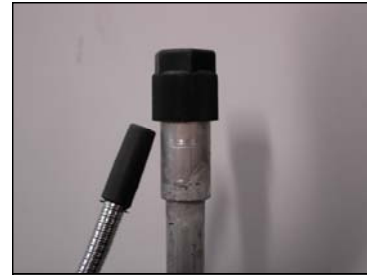
Figure 4.22.b. Detection from the bottom of a R-134a leak from a MAC system fitting, using a 7 g.yr -1 sensitivity threshold – detector.
