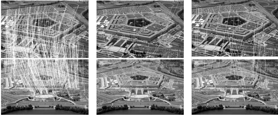
Figure 6.28: Pentagon, with transition tilt \tau \approx 2.5 . ASIFT (shown), SIFT (shown), Harris-Affine, Hessian-Affine and MSER (shown) find respectively 378, 6, 2, 8 and 17 correct matches.
