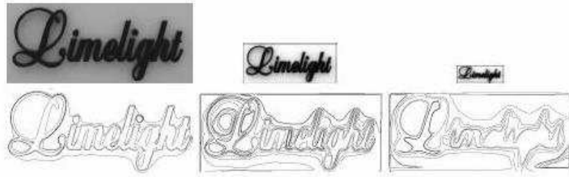
Figure 6.10: Top: the same shape at different scales. Bottom: Their level lines (shown at the same size). The level line shape changes with scale (in other terms, it changes with the camera distance to the object).
