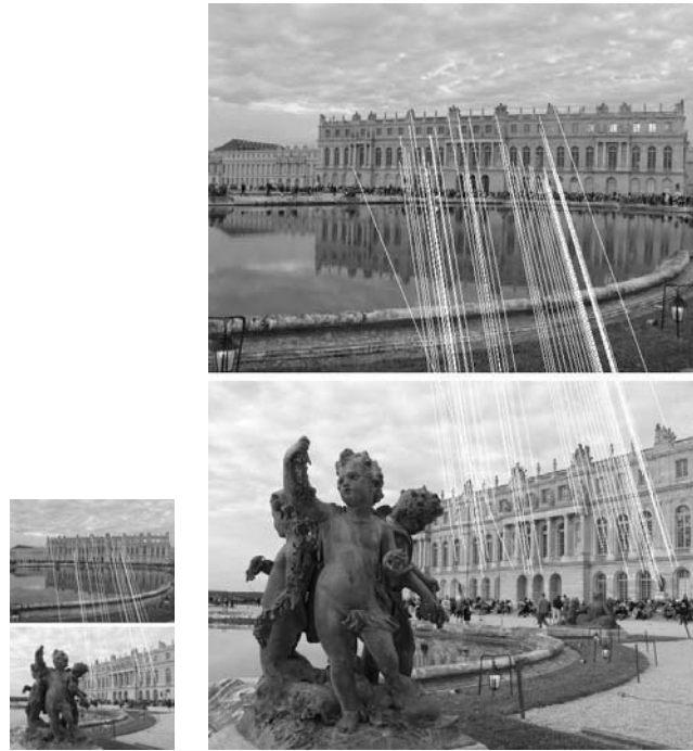
Figure 6.15: Two-resolution ASIFT. Left: low-resolution ASIFT applied on the 3 \times 3 subsampled images finds 19 correct matches. Right: high-resolution ASIFT finds 51 matches.
