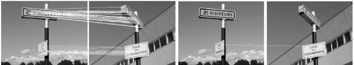
Figure 6.27: Image matching: road signs. Transition tilt \tau \approx 2.6 . ASIFT (shown), SIFT, Harris-Affine, Hessian-Affine and MSER (shown) find respectively 50, 0, 0, 0 and 1 correct matches.
