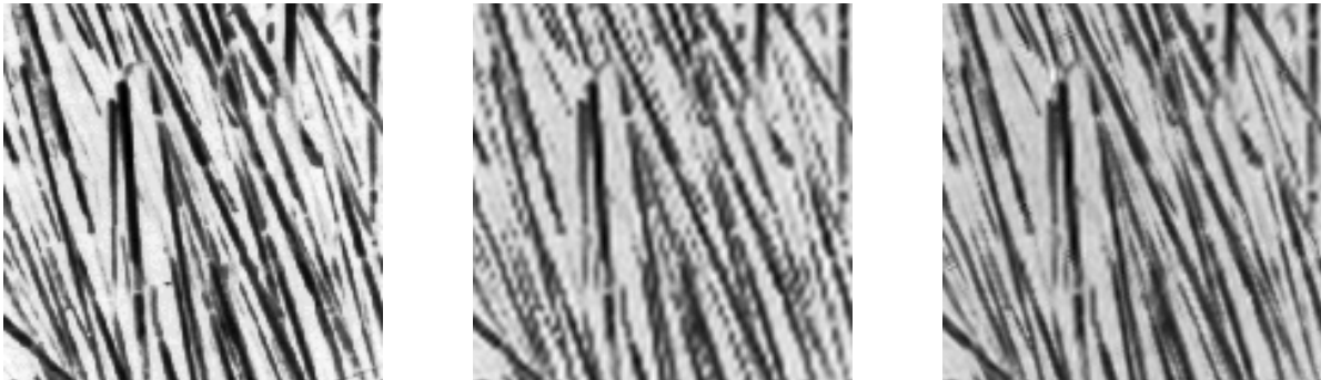
Figure 1.4: Left: High-resolution image. Middle: Cubic spline interpolation 21.37 dB. Right: Super-resolution 23.82 dB
