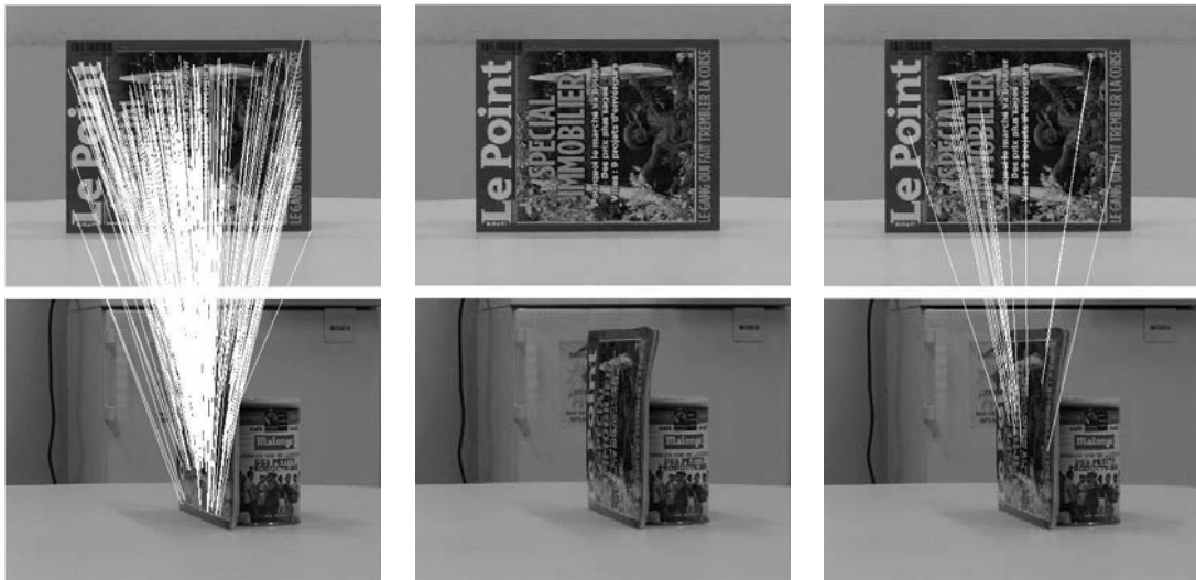
Figure 6.24: Correspondences between magazine images taken with zoom \times 4 , frontal view and 80° angle, absolute tilt t \approx 5.8 . ASIFT (shown), SIFT (shown), Harris-Affine, Hessian-Affine, and MSER (shown) find respectively 349, 0, 0, 0, and 17 correct matches.
