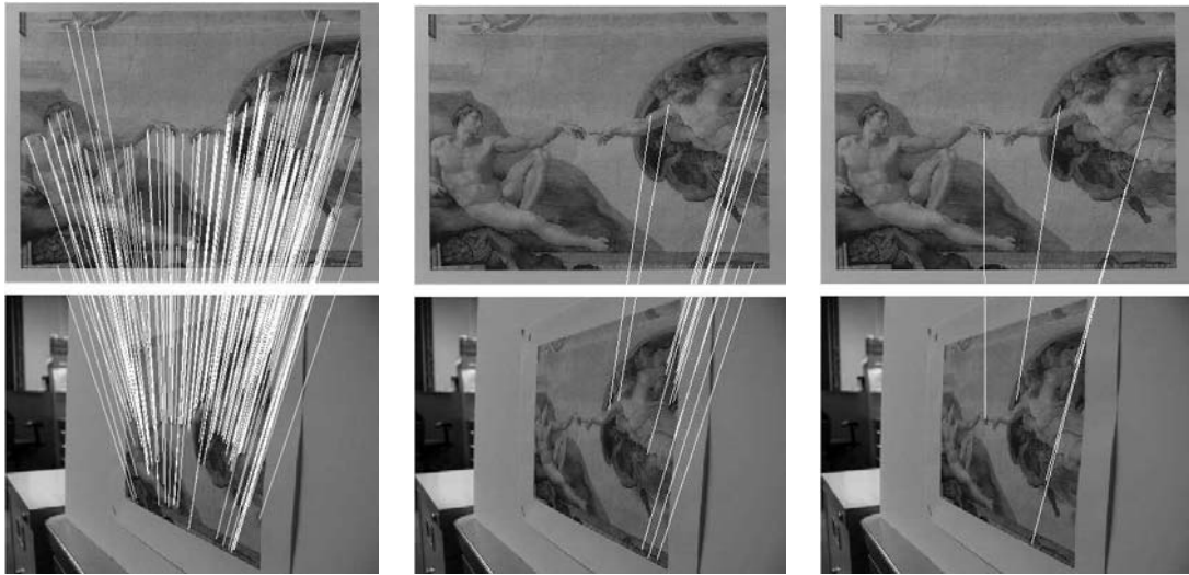
Figure 6.22: Correspondences between the painting images taken from short distance (zoom \times 1 ) at frontal view and at 75^\circ angle. The local absolute tilt varies: t \approx 4 (middle), t < 4 (right part), t > 4 (left part). ASIFT (shown), SIFT (shown), Harris-Affine, Hessian-Affine, and MSER (shown) find respectively 202, 15, 3, 1, and 5 correct matches.
