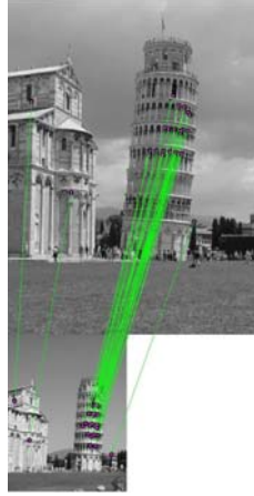
Figure 5.1: A result of the SIFT method, using an outliers elimination method [170]. Pairs of matching points are connected by segments.
