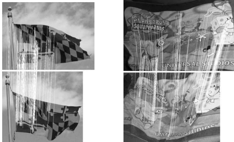
Figure 6.30: Image matching with object deformation. Left: flag. ASIFT (shown), SIFT, Harris-Affine, Hessian-Affine and MSER find respectively 141, 31, 15, 10 and 2 correct matches. Right: SpongeBob. ASIFT (shown), SIFT, Harris-Affine, Hessian-Affine and MSER find respectively 370, 75, 8, 6 and 4 correct matches.
