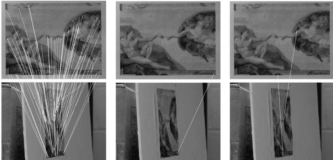
Figure 6.23: Correspondences between long distance views (zoom \times 10 ), frontal view and 80^\circ angle, absolute tilt t \approx 5.8 . ASIFT (shown), SIFT, Harris-Affine (shown), Hessian-Affine, and MSER (shown) find respectively 116, 1, 1, 0, and 2 correct matches.
