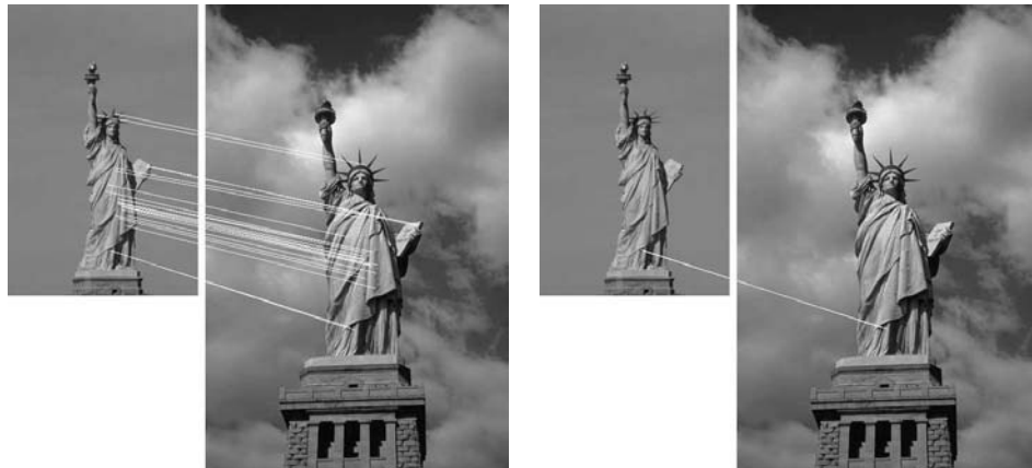
Figure 6.29: Statue of Liberty, with transition tilt \tau \in [1.3, \infty) . ASIFT (shown), SIFT (shown), Harris-Affine, Hessian-Affine and MSER find respectively 22, 1, 0, 0 and 0 correct matches.
