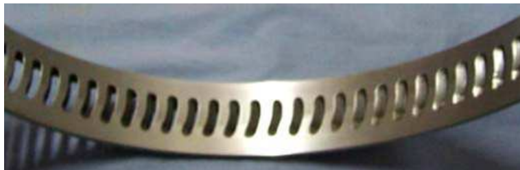
Figure 1.9: Example of casing treatment. From Jiang[79].
