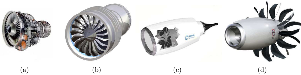
Figure 1.3: Snecma and CFM jet engines. (a) CFM 56. (b) Leapx. (c) Contrarotative fan. (d) Open rotor.
