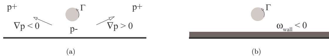
Figure D.2: (a) Pressure gradients induced by the vortex. (b) Schematic of the vorticity layer induced at the wall by the no-slip boundary condition.
