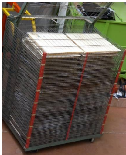
Figure II.30 - Claie de séchage.
