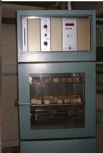
Figure II.6-Séchage des cubes.
