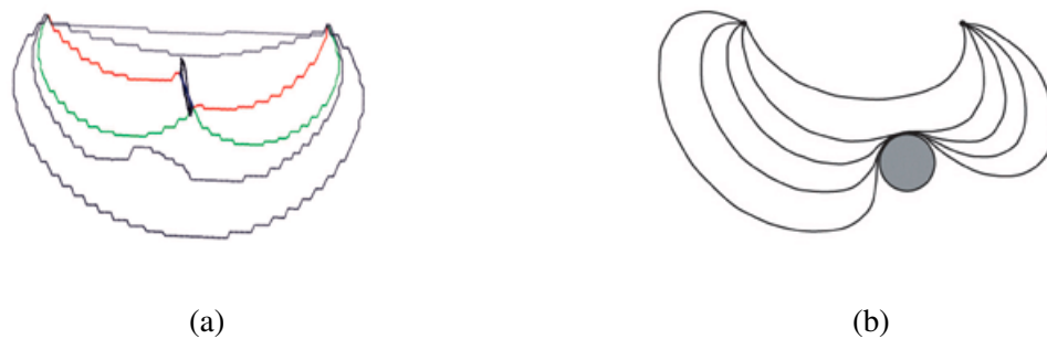
Figure 17 - Successive snapshots of (a) a lattice-based simulation ("pure-mixed" model, mM code) of a dislocation-dislocation interaction [MicroMégas], and (b) a nodal simulation of a dislocation-precipitate interaction [Douin].
