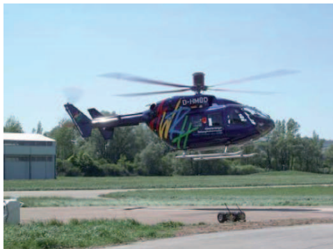
Figure 1.5: BK117 with PZT actuated TEF to perform secondary control. (Ref. [4])
