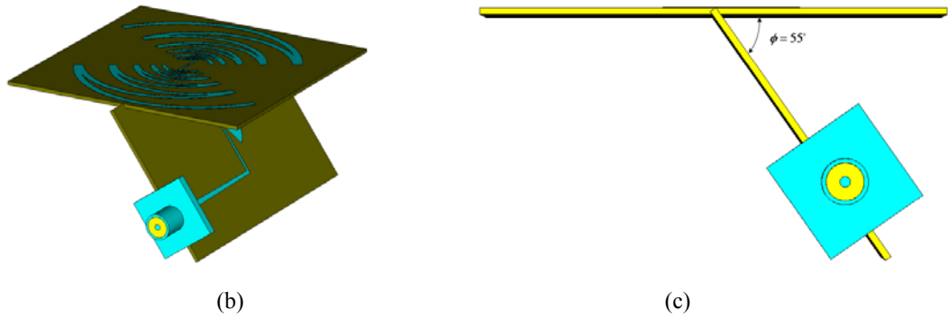
Fig.3.32. (Continued) (b), (c) Sinuous antenna connected to the balun geometry in second form.
