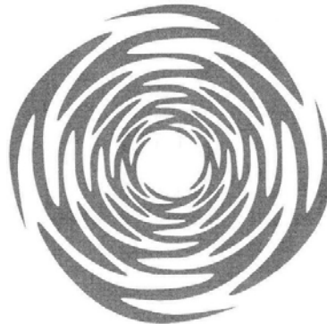
Fig.1.5. The sinuous antenna geometry.
