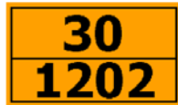
Figure 31. Example of a code of danger sign for dangerous goods, in accordance with the Kemler code.
