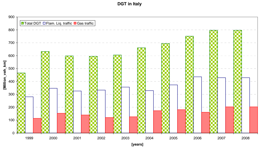
Figure 24. Comparison between the total amount of dangerous goods, flammable liquids, and gases – respectively -transported in Italy, expressed in [million veh · km ] - (“Panorama of Transport”, 2009) and (“Annual road freight transport of dangerous goods, by type of dangerous goods and broken down by activity”, 2010).
