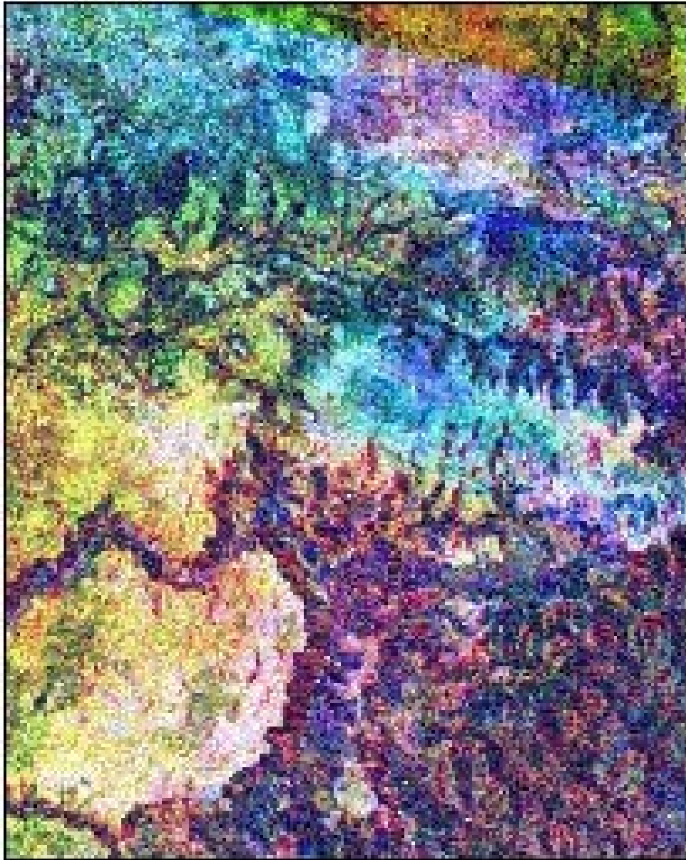
Figure 2: False colors composite of the coherence extracted from July (cp07: Red), August (cp08: Green) and February (cp02: Blue) acquisitions. Grasslands and bushlands appear as white or light tones, the darker tones being forest.
