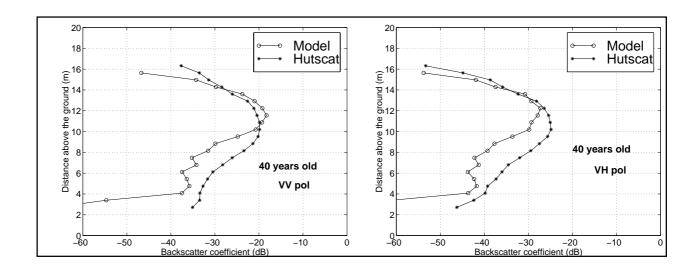
Fig. 10 : Comparisons between experimental and simulated profiles for a 40 years old stand at X band, VV and VH polarization in the near normal incidence mode.
