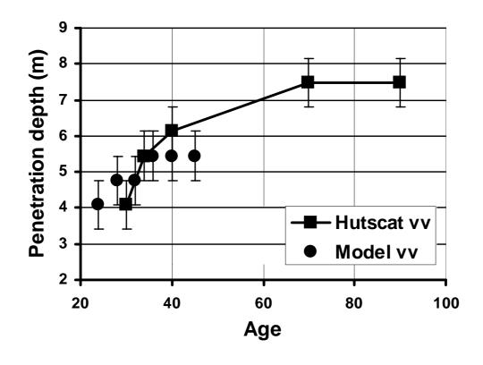
Fig. 12 : Simulated and experimental penetration depths at X band near normal incidence as a function of the age of the stand. The penetration depth  $\delta_p$  is the depth at which  $I(\delta_p)/I(0)=1/e$ , I(0) being the transmitted intensity of the incident wave.
