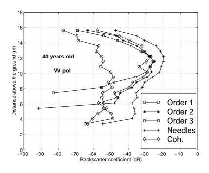
Fig. 11: Absolute contributions (in dB) of the simulated vertical backscatter profiles for each vegetation element of each layer, for a 40 years old pine stand at X VV channel in the near normal incidence mode.
