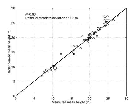
Fig. 5: Radar derived mean height versus the in-situ measurements for 66 samples plots of Austrian Pine. Results are presented for the X band HH channel.
