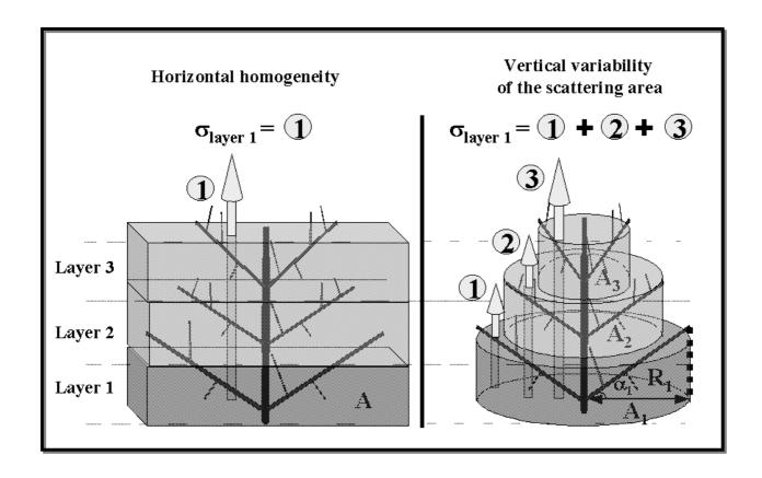
Fig. 7: 3- layer medium describing a crown using two approaches: (left) the scattering area is an infinite homogeneous layer, (right) the scattering area is defined as the disk for which the radius depends on the mean length of the primary branches belonging to the layer.
