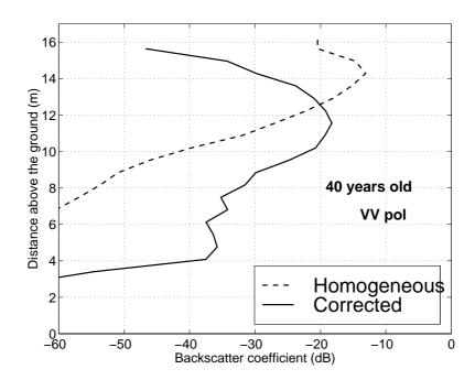
Fig. 8 : Vertical backscatter profiles using the actual scattering area correction ("corrected") and the infinite layer hypothesis ("homogeneous"). Results are presented for X band at VV polarization for a 40-year old Austrian pine at  $3^{\circ}$  incidence.
