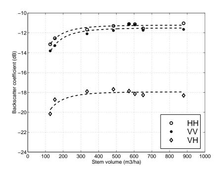
Fig. 4: Crown backscatter of Austrian pine stands, for the near-normal incidence mode, and for the 3 polarizations at X band versus the stem volume. The crown backscatter is the sum of all the contributions coming from all the resolution cells in the radar backscatter profiles within the crown.
