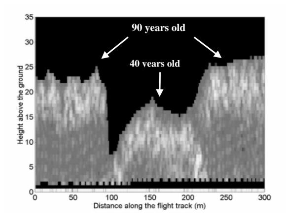
Fig. 2: Succession of 300 vertical backscatter profiles measured by HUTSCAT at X band and HH polarization, along a transect over 3 Austrian pine stands of (from left to right) 90, 40 and 90 years old. A profile is measured at each meter, and the vertical resolution is of 0.68 cm. The different tones denote the backscatter intensity of each resolution cell.
