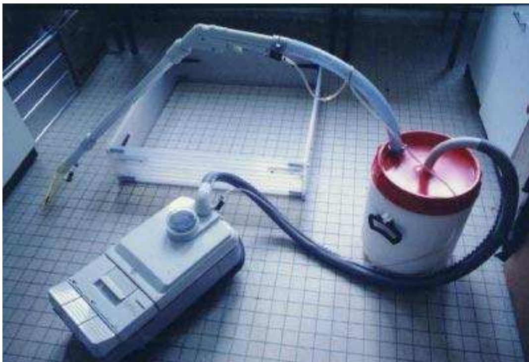
Fig. 1 Floor and carpet vacuum cleaner modified for urban deposit sampling : domestic cleaner for floor and carpet (Kärcher model 555 c) and high density polyethylene vessel (34 l). Street deposit sampling area is determined by a 80 × 80 cm plastic frame : here the studied surface is a University laboratory floor covered with dried and sieved sediments
