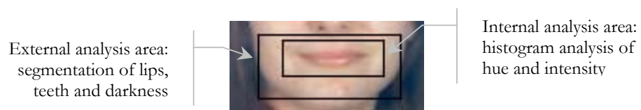
Figure IV-28. Areas delimited for the histogram study and for the mouth motion analysis
