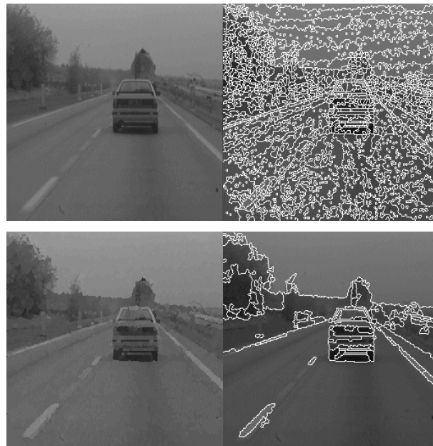
Figure App-5. Top: Initial image (left) and initial watershed of the gradient (right). Bottom: Mosaic image (left) and first level of hierarchy (right).
