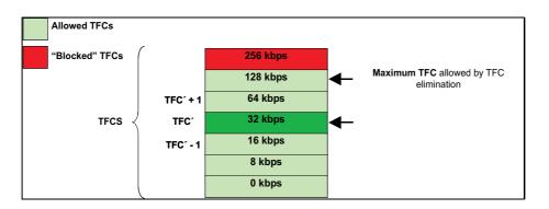
Figure 4.10: Transport Format Combination Selection Procedure.
