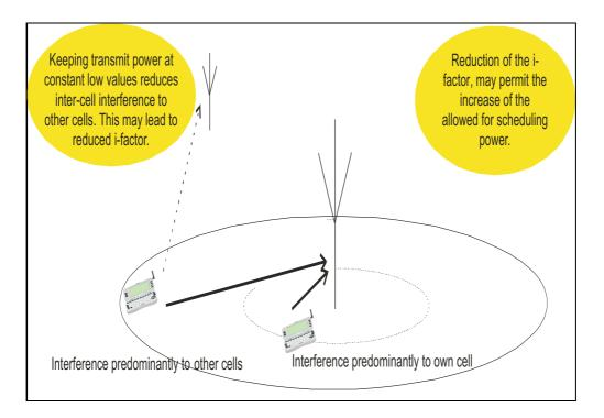
Figure 5.1: Basic concept of the fast VSF scheme.
