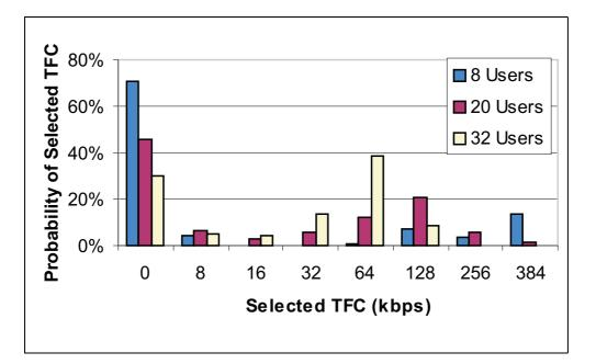
Figure 4.22: Probability of selected TFC for the cases of 8, 20 and 32 users per cell.
