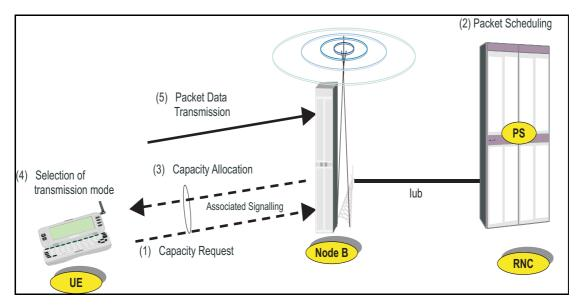
Figure 1.2: Principle of the uplink packet access in UTRAN.
