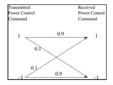
Figure A.1: Model of errors of the power control command
