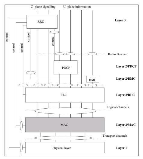
Figure 2.1: Radio Interface Protocol Architecture in UTRAN.
