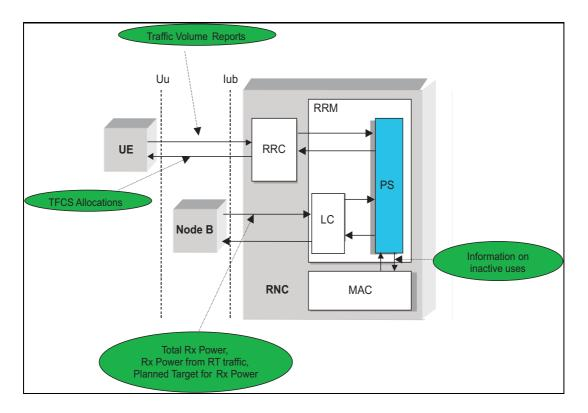
Figure 4.4: Packet Scheduling Working Environment (figure inspired from corresponding figure in [40]).
