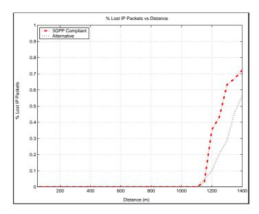
Figure 3.7: Percentage of lost IP packet for various distances between the UE and the Node B.
