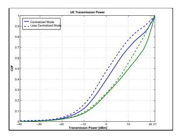
Figure 5.11: CDF of the UE transmission power, for the cases of the centralized and decentralized schemes.
