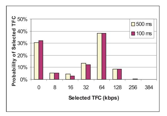
Figure 4.12: Probability of selected TFC for all of the users in the system (TFC Elimination "On and "Off", 8 users per cell, cell radius 933 m).
