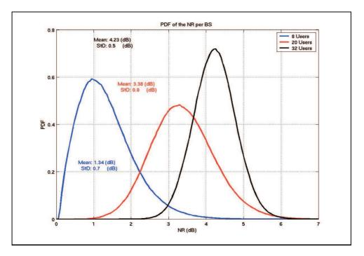
Figure 4.23: PDF of the noise rise for the cases of 8, 20 and 32 UEs per cell.
