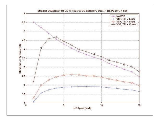
Figure B.3: Standard deviation of the UE transmission power versus UE speed for the cases the fast VSF is deactivated and activated.
