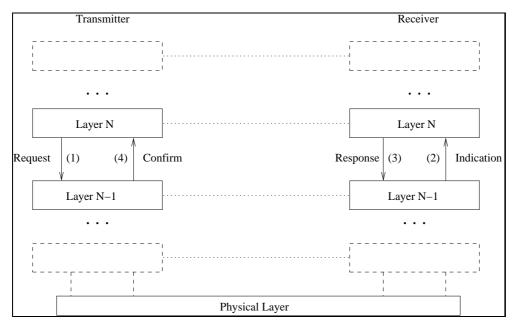
Figure 3.1: Use of the four types of primitives. The numbers next to the primitive names indicate the order of their transmission.
