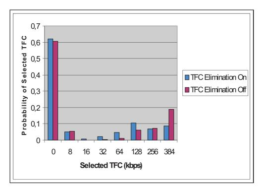
Figure 4.15: Probability of selected TFC for all of the users (TFC Elimination "On and "Off", 8 users per cell, cell radius 1866 m).
