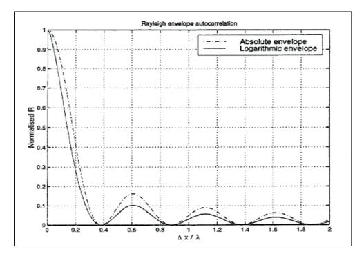
Figure B.2: Envelope autocorrelation of fast fading in Clarke's scattering model ([55]).
