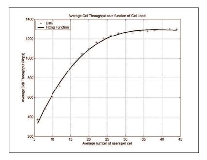
Figure 4.21: Mean Cell Throughput for different number of UEs in the cell.
