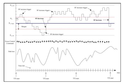
Figure 5.3: Implementation of the fast VSF scheme.
