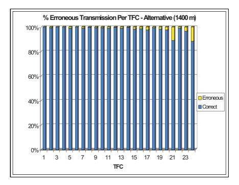
Figure 3.12: Percentage of correct-erroneous reception per selected TFC in the case of the alternative TFC selection algorithm.
