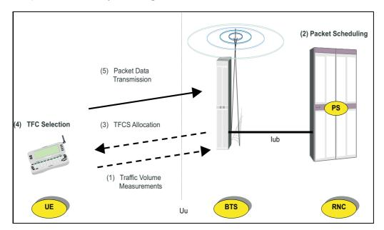
Figure 4.2: Overview of the Uplink Packet Data Access in WCDMA Uplink
