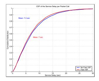
Figure 5.6: CDF of the experienced delay per packet call (fast VSF "On" and "Off", 12 UEs per cell, traffic model scenario B).
