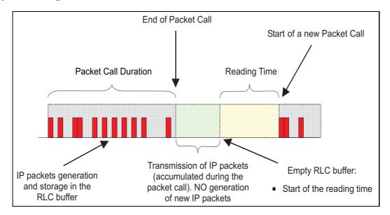
Figure 4.11: A simple modeling approach to include closed loop transmission model.
