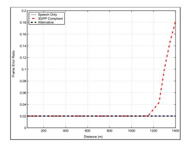
Figure 3.5: FER for various distances between the UE and the Node B.
