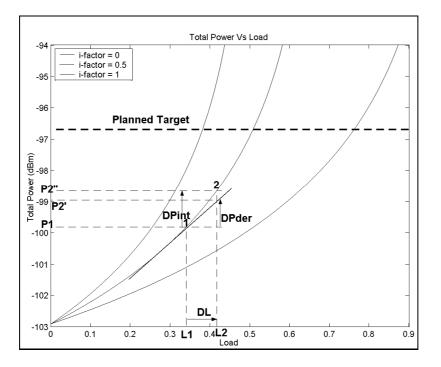
Figure 4.8: Estimation of the new total received power due to the change of the load of a user.
