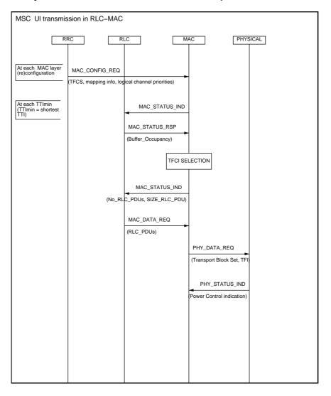
Figure 3.4: Uplink transmission in MAC layer in dedicated mode (UE side).
