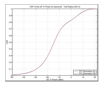
Figure 4.13: CDF of the UE transmission power (TFC Elimination "On and "Off", 8 UEs per cell, cell radius 933 m).
