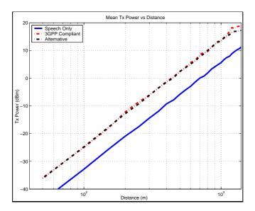
Figure 3.8: Mean UE transmission power for various distances between the UE and the Node B.
