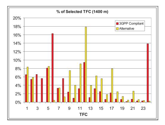
Figure 3.9: Probability of selected TFC for a distance to the Node B equal to 1400 m.
