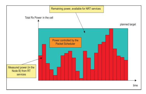
Figure 4.1: Division of the total received (Rx) power in uplink between RT and NRT traffic.
