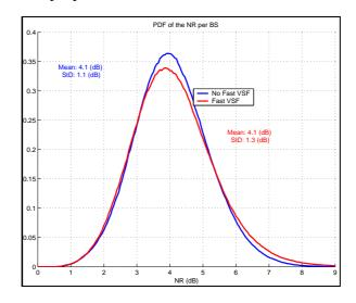
Figure 5.5: PDF of the noise rise (fast VSF "On" and "Off", 12 UEs per cell, traffic model scenario B).
