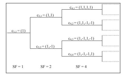
Figure 2.4: Code generation tree of the orthogonal variable spreading codes used in UTRAN.
