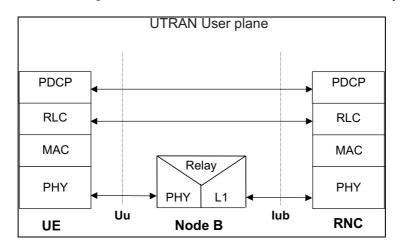
Figure 2.2: User Plane protocol stack in the case of establishment of dedicated channels between the UE and the network.
