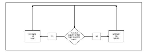
Figure A.3: General Model of the outer loop power control.
