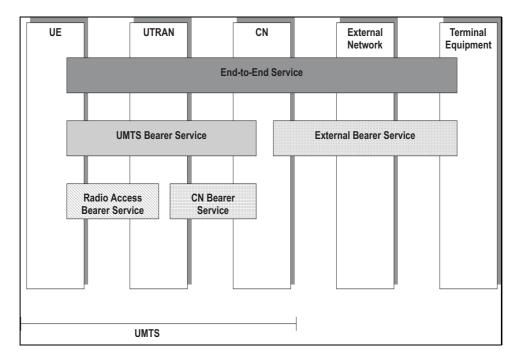
Figure 1.3: Simplified Overview of the layered QoS architecture in UMTS.
