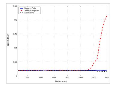
Figure 3.6: Speech BLER for various distances between the UE and the Node B.
