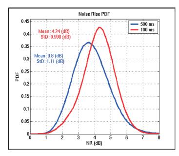
Figure 5.14: PDF of the noise rise, for the cases the packet scheduling period is 500 and 100 ms (12 UEs per cell, traffic model scenario B).
