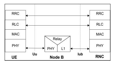
Figure 2.3: Control Plane protocol stack when dedicated channels are established between the UE and the network.
