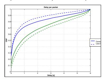
Figure 5.10: CDF of the experienced delay per IP packet, for the cases of the centralized and decentralized schemes (10 UEs per cell).
