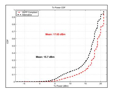
Figure 3.10: CDF of the UE transmission power for a distance to the Node B equal to 1400 m.
