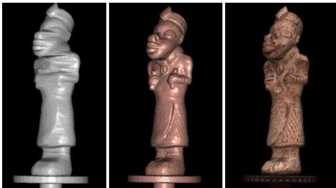
Figure 3.5: Complete reconstruction sequence of the BigHead object. From left to right: visual hull, snake after convergence and texture mapping. The reconstructed model has 114496 vertices.
