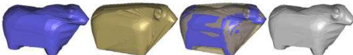
Figure 3.51: Visual hulls computed with both sequences after registration. From left to right: visual hull of the first sequence, visual hull of the second sequence, superposition of both visual hulls and intersection of both visual hulls.
