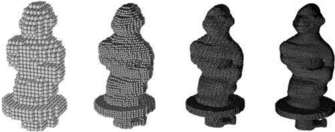
Figure 2.7: Octree construction of a visual hull. From left to right, the level of detail ranges from 5 to 8 depth levels.
