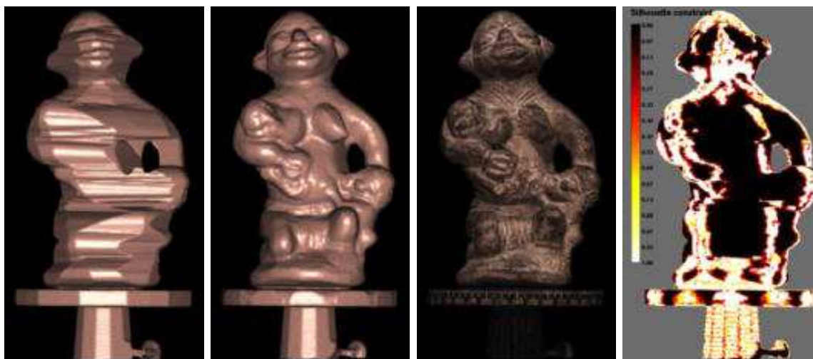
Figure 3.12: Twins model reconstruction using only 12 equally spaced cameras. From left to right: visual hull initialization, final model, texture mapping, and concavity recovery.
