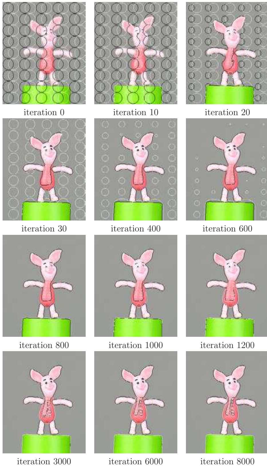
Figure A.14: 4-phase segmentation using the proposed speed. The level sets are able to converge to the global minimum. \phi_0 and \phi_1 zero level set are drawn in black and white color, respectively.
