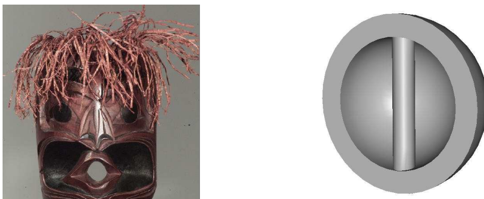
Figure 2.3: Example of objects whose topology cannot be correctly captured by the visual hull concept.
