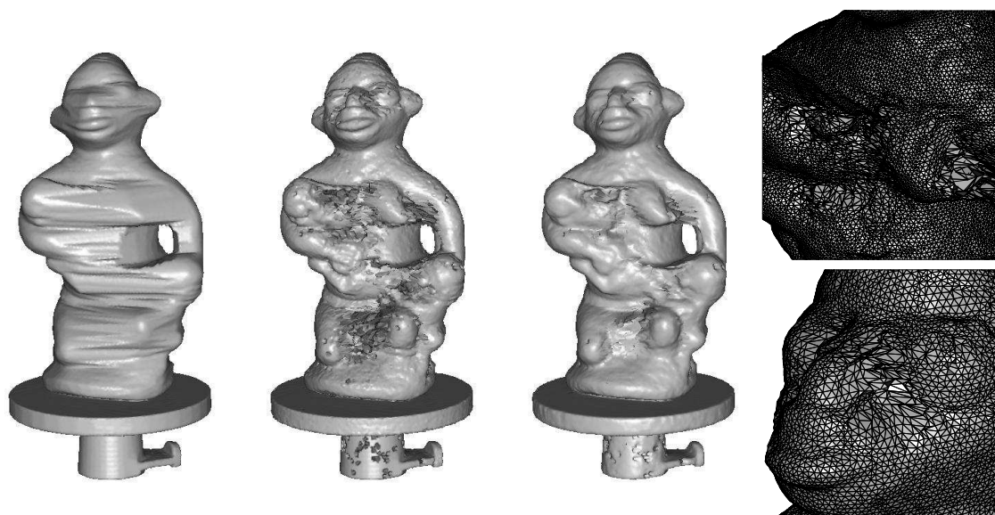
Figure 2.16: Reconstruction of the Twins object by local vertex optimization using multi-correlation. From left to right: visual hull, deformed model, filtered model and detail of some reconstruction errors of the filtered model.
