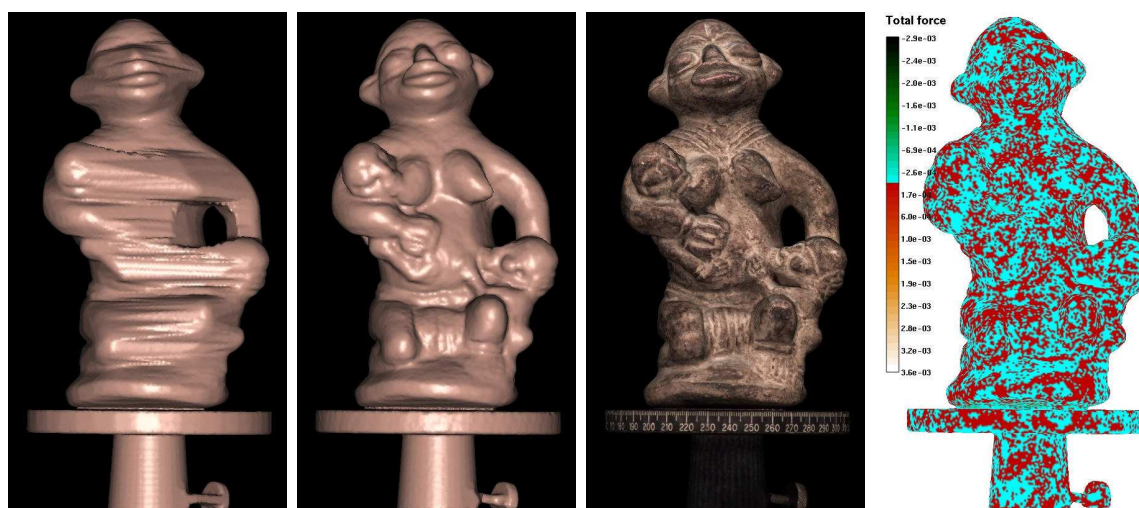
Figure 3.10: Different steps in the reconstruction process of the Twins object. From left to right, visual hull initialization, final model, texture mapping and total force after convergence. The reconstructed model has 83241 vertices.
