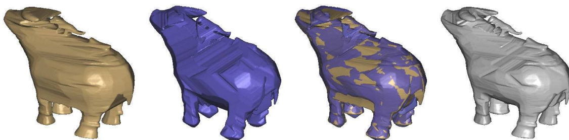
Figure 3.57: Visual hulls of the two silhouette sequences after registration. The final mutual coherence is of 95%. From left to right: visual hull of the first sequence using 36 silhouettes, visual hull of the second sequence using 8 silhouettes and both visual hulls superposed.
