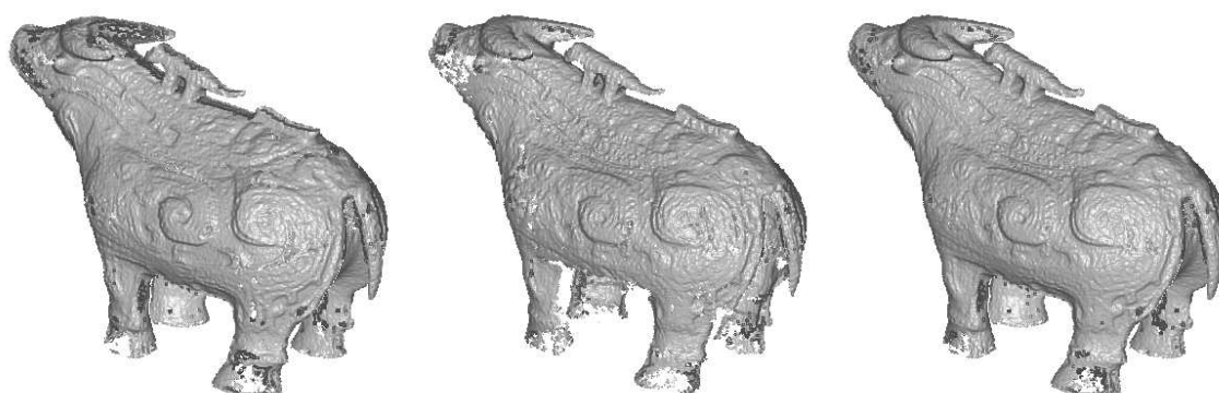
Figure 3.58: From left to right, correlation volumes corresponding to the first sequence, the second sequence and the two volumes mixed. All the volumes have been binarized with a threshold of 30.
