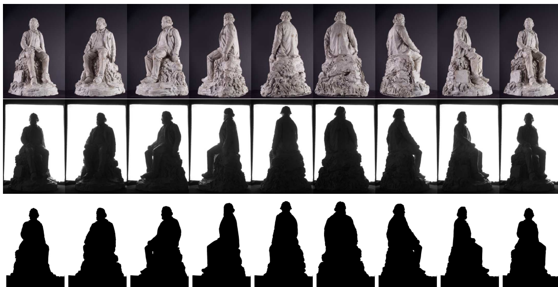
Figure 3.35: Some of the original images used in the reconstruction of the Millet object. Top: 9 samples of a total of 36 color images. Bottom: 9 samples of a total of 36 silhouette images.
