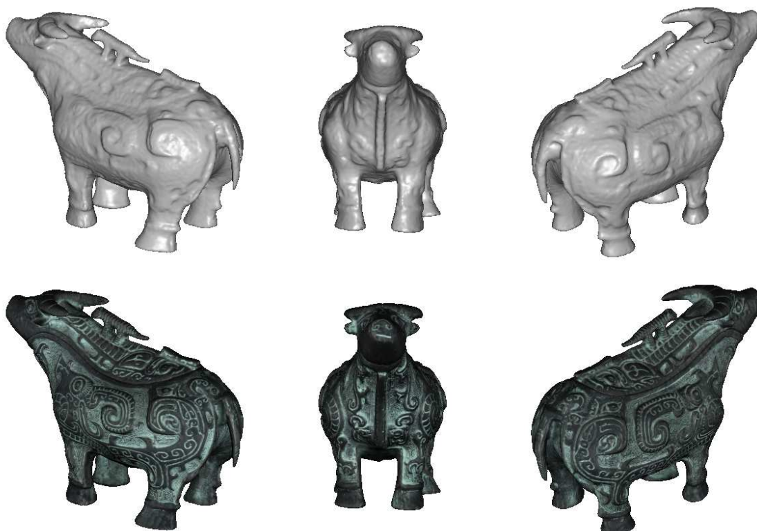
Figure 3.61: Final Buffle model with 58734 vertices. Top: 3 shaded views. Bottom: the same views with texture mapping.
