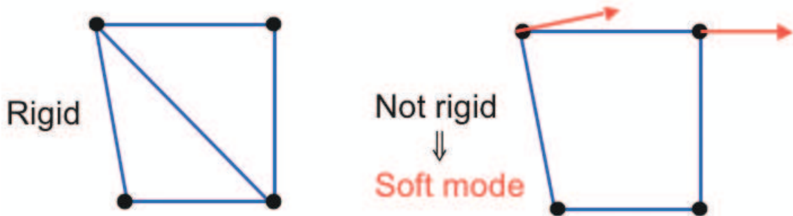
Fig. 2.1: Illustration of a rigid and a floppy network made of 4 particles interacting with springs. Nd - d(d+1)/2 = 5 contacts are required to rigidify the structure. The red arrow of the floppy network indicates the soft mode that appears when one contact from the rigid system is removed.
