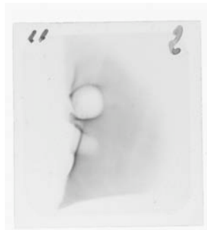
Figure 3.30: Double-Bubble structures observed in some shots. Here the proton image has been obtained with N_2 gas at 50 at \approx 28.8 ps after the arrival of the main laser beam on the electron target (i.e. they are formed by protons with \approx 3.1 MeV energy).
