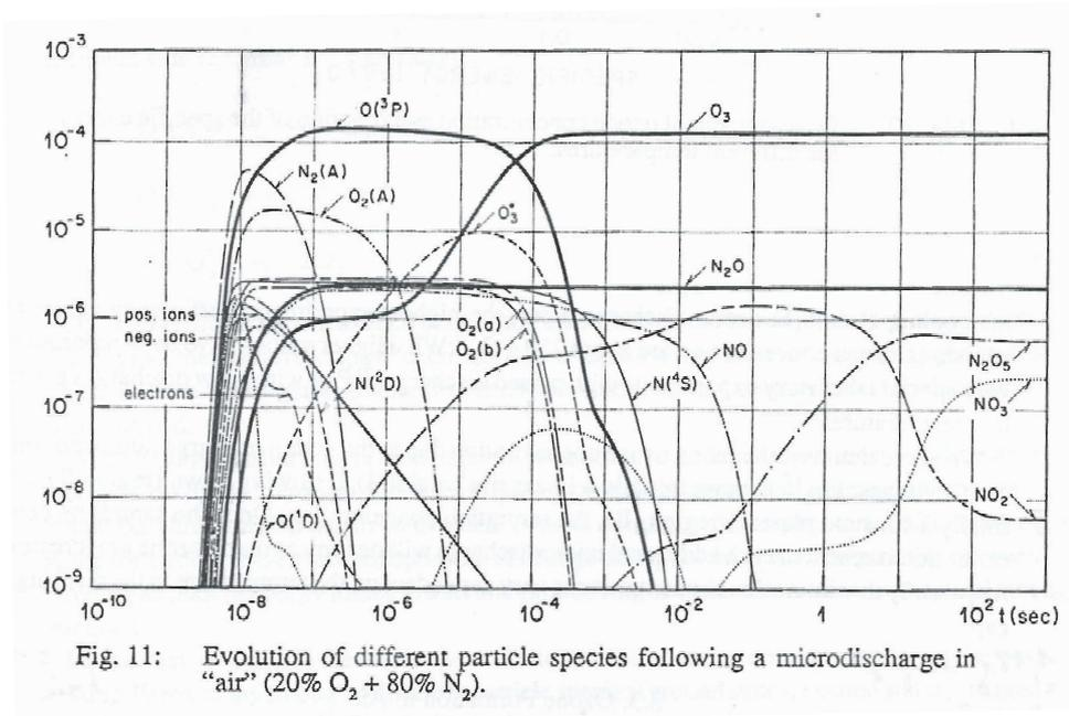
Fig. 11: Evolution of different particle species following a microdischarge in "air" (20% O<sub>2</sub> + 80% N<sub>2</sub>).
