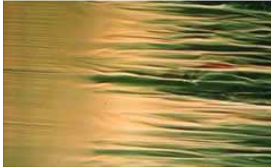
Figure 1.3: Boundary-layer transition on the surface of a flat plate, seen from the top. Flow is from left to right and dye visualization shows the transition from laminar (on the left) to turbulent flow (on the right). (Photograph courtesy of ONERA)
