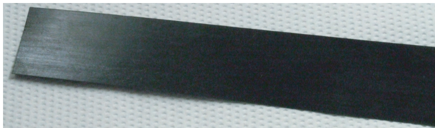
FIGURE 3.13 – Ruban de composite APC-2
