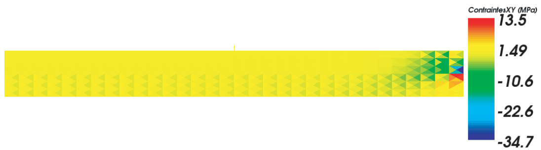
FIGURE 4.33 – Champ de contraintes \sigma_{XY} à t=10 s
