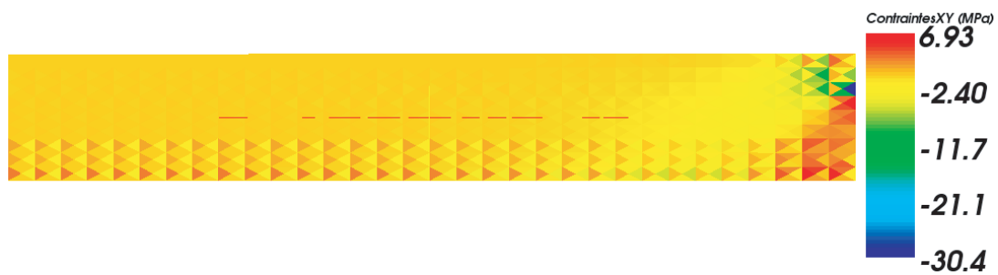
FIGURE 4.74 – Champ de contraintes \sigma_{XY} à t=10 s
