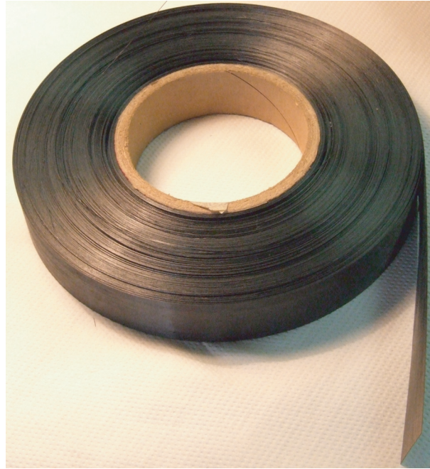
FIGURE 3.12 – Rouleau de composite APC-2
