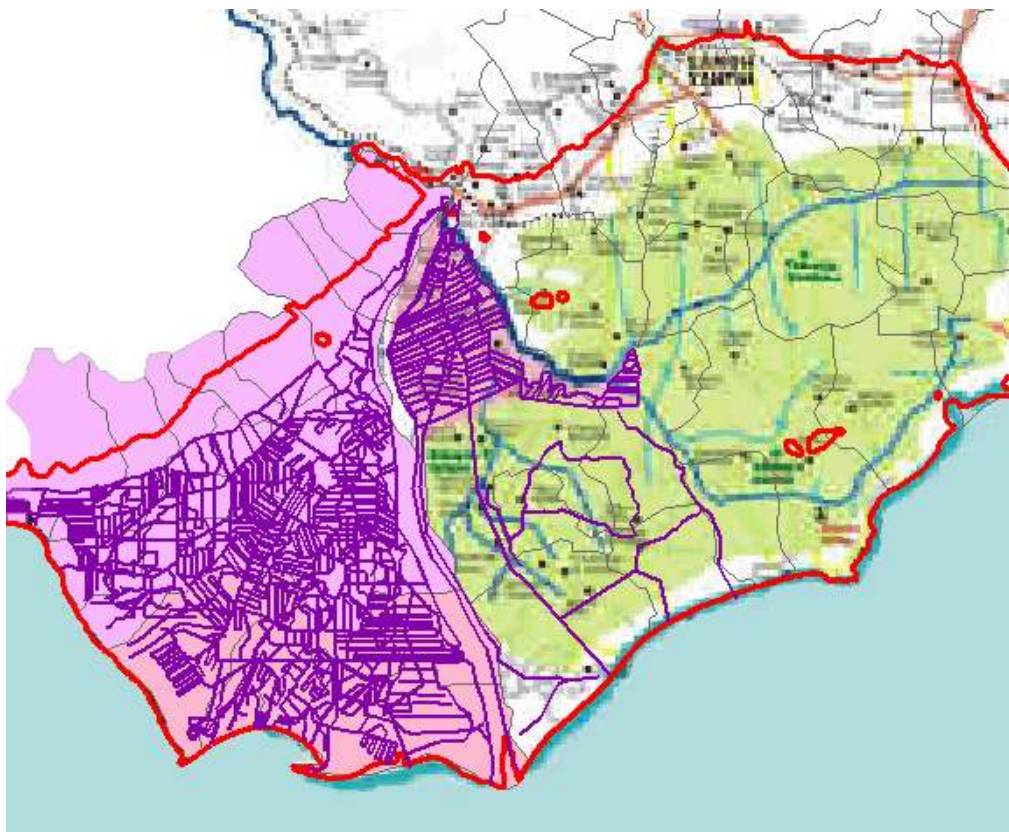
Figure 91 - Present irrigation system in the Nestos delta (in pink-magenta) and future extension to the Xanthi plain (in green-blue) in liaison with the Temenos dam project
