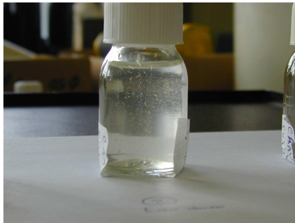
Fig. 2 Production of fines picture in water effluent for CR reservoir core
