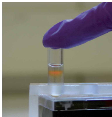
Figure 3 | Picture of the QD band after 25 min ultracentrifugation in 30% sucrose at 300,000g.
