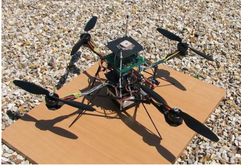
FIGURE 6.1. Our home-built quadrotor: the “Quadricopter”.
