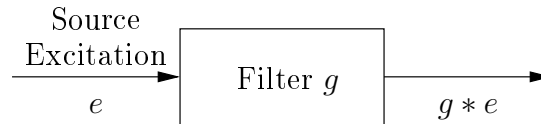
Figure 3.4: Source/Filter model: the glottal source excitation e is filtered by filter g , leading in the time domain to the convolution g * e .
