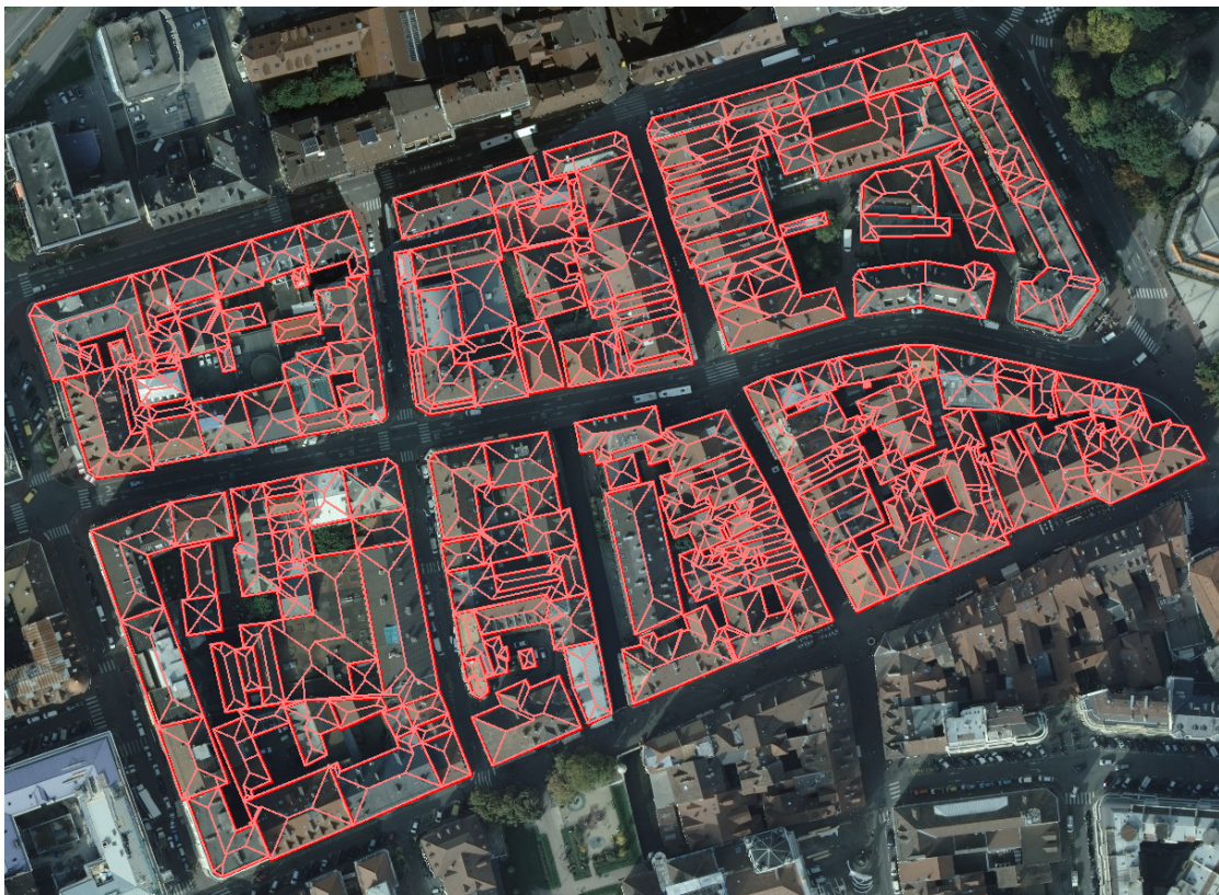
Figure 7.3: Straight Skeleton-based Reconstruction
