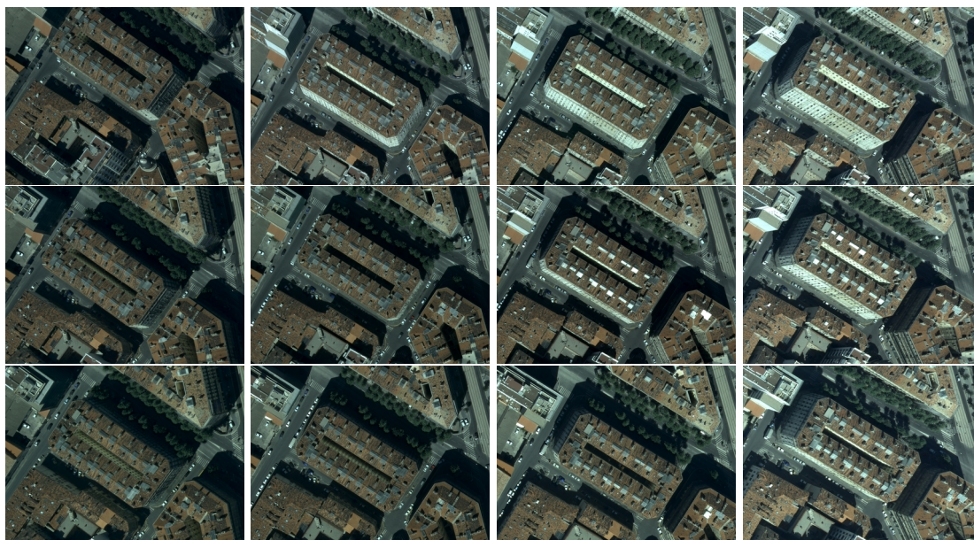
Figure 2.2: 1186x880 convergent image crops showing the same building viewed from 12 different airplane locations. Each uncropped image has 13824x7680 pixels.
