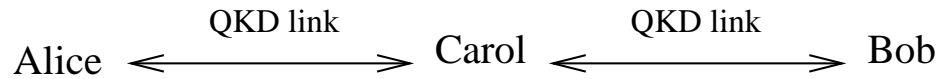
Figure 10.3: QKD bridge: Alice and Bob are out of the QKD range; they want to use Carol as a bridge to communicate securely the session key.
