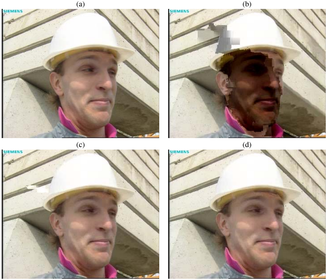
Fig. 11. 5-th image of Foreman.cif obtained after (a) error-free decoding, (b) standard decoding, (c) robust decoding, and (d) CRC-robust decoding for a SNR of 2.8 dB and a MAC payload size of 120 bytes, with channel coding.
