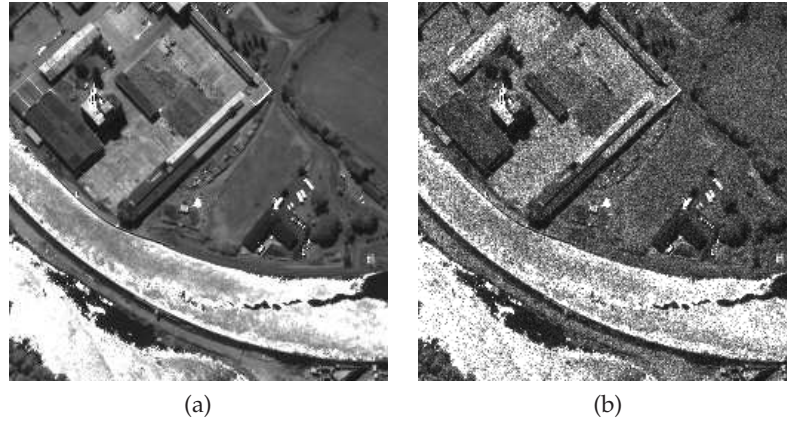
FIGURE 20 – Optical image with simulated 3-look speckle noise : original (a) and noisy image (b).
