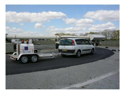
Fig. 3-2 HWD test on the LCPC's fatigue carrousel test facility (photograph by M Broutin)
