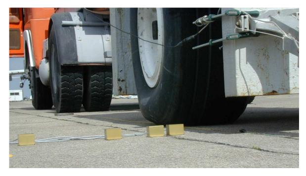
Fig. 0-14 STAC's inclinometer system, zoom view (Photograph by D. Guédon, Toulouse LRPC)
