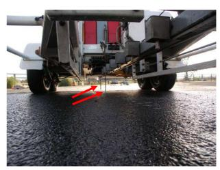
Fig. 3-3 Assisted positioning system over gages profiles (photographs by M. Broutin)
