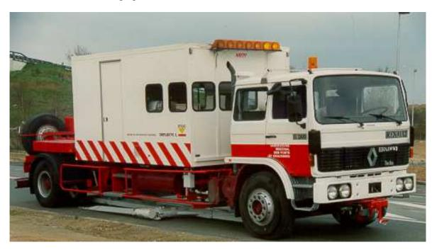
Fig. 0-15 The Lacroix Deflectograph (source: LCPC's database)
