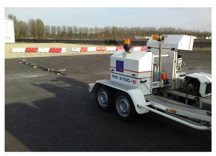
Fig. 1-43 Test setup to measure long radial distances deflections
