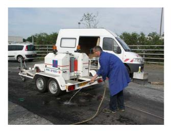
Fig. 3-4 Continuous spraying of the surface pavement during the whole tests series duration (Photograph by M. Broutin)
