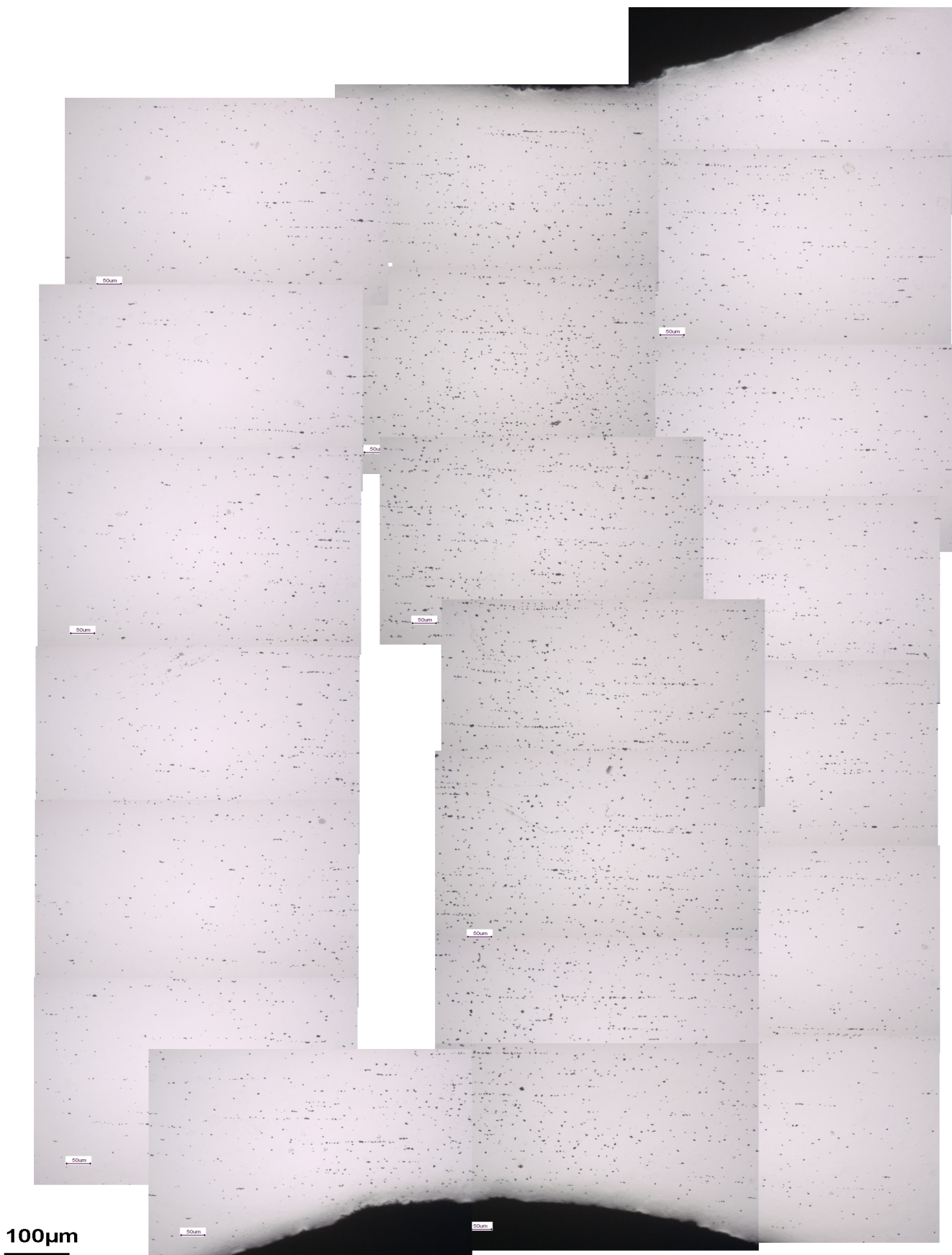
Figure VII.52 : Creep damage in one unbroken notch of the NTDC1.2 notched specimen interrupted after 14,137h of creep at \sigma_n = 170\text{MPa} , 600^\circ\text{C}
