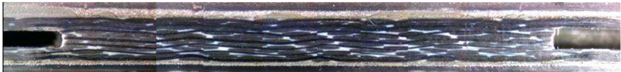
Figure X.12 – Echantillon Arcan-Mines poli miroir avant essai
