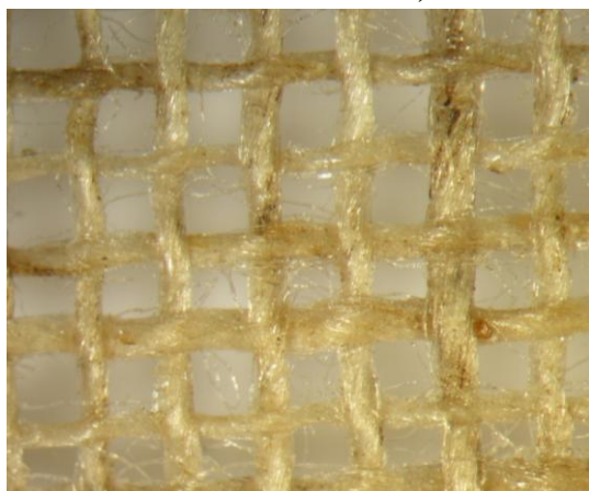
Figure 135 : élimination de la Beva®, \lambda : 248 nm, F = 1,12 J/cm 2 .10 pulses, Ablation +++
