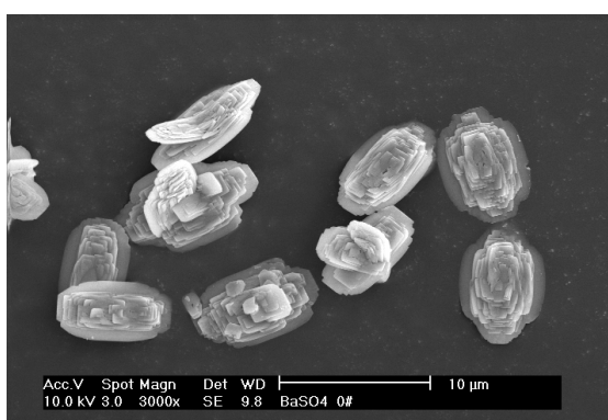
Fig.3.29 SEM image of \text{BaSO}_4 formed in the absence of inhibitor ( \times 1500 )
