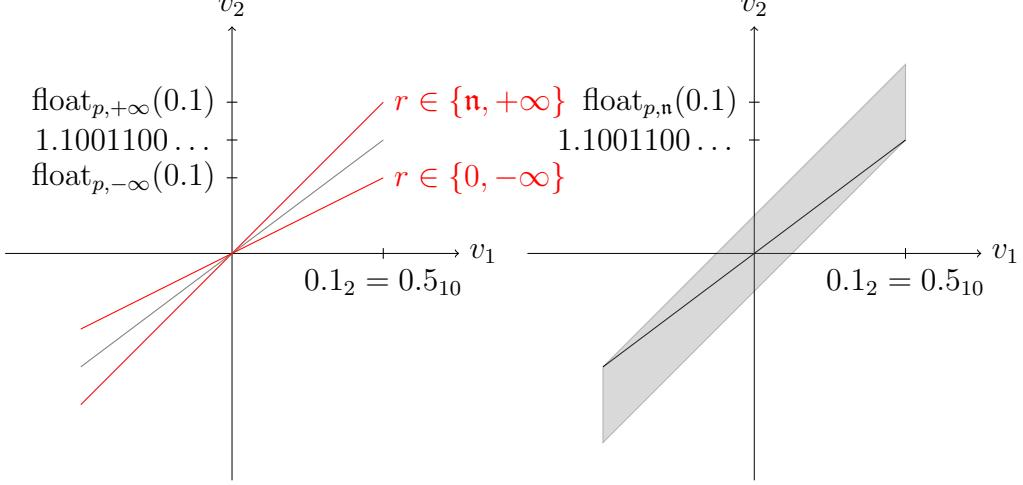
Figure 7.1: Unsafe approximation of affine sets: the correlation is falsified by the use of floating-point numbers.
