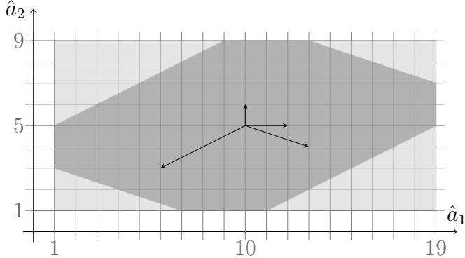
Figure 3.1: The joint range (the center symmetric polygon in dark gray) of two affine forms. This zonotope is spanned by the generators drawn in its center. The box  $\hat{\mathbf{a}}_1 \times \hat{\mathbf{a}}_2$  (light gray) encloses the zonotope.
