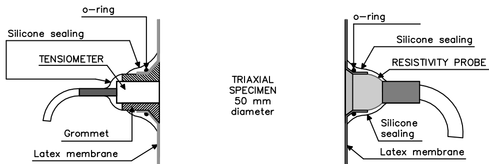
Figure 7. Triaxial specimen. Lateral view. Holding system for the tensiometer (left) and the resistivity probe (right)
